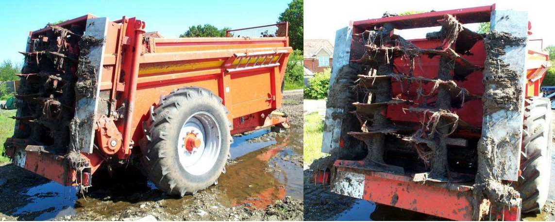
Figure 2. Rear discharge FYM spreader.
