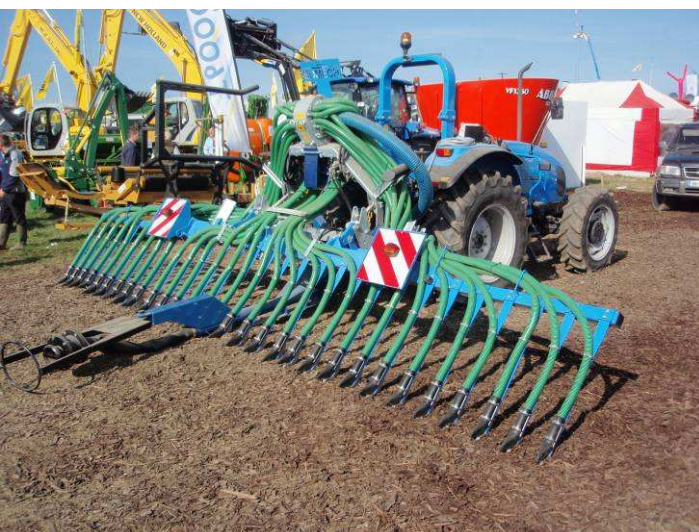
Figure 4. Umbilical system spreader
