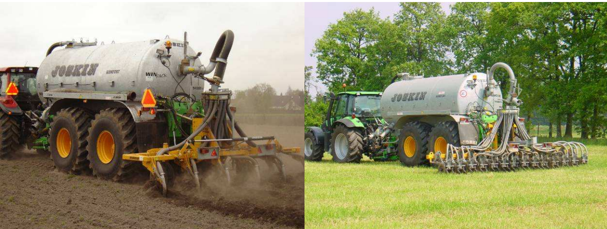
Figure 3. Equipment for injecting slurry into soil and pasture.
