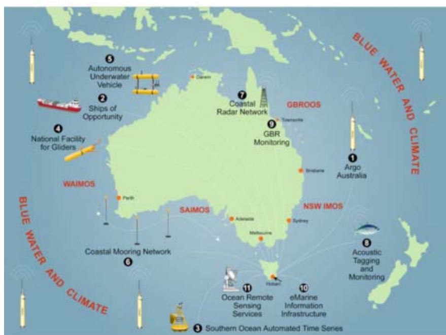
Figure 4. Schematic of Australia's Integrated Marine Observation System (IMOS). See imos.aodn.org.au for more information.
