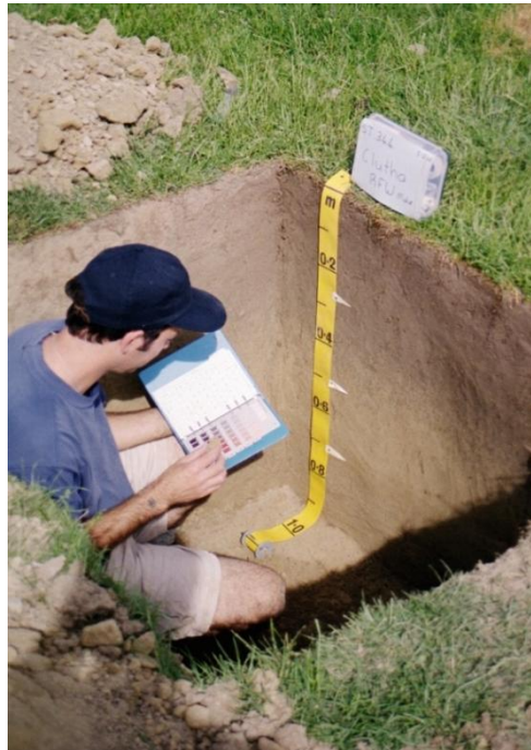
Figure 1 Sam Carrick describing the morphology of a soil profile exposed in a pit prior to sampling the soil horizons, at a site in Southland
