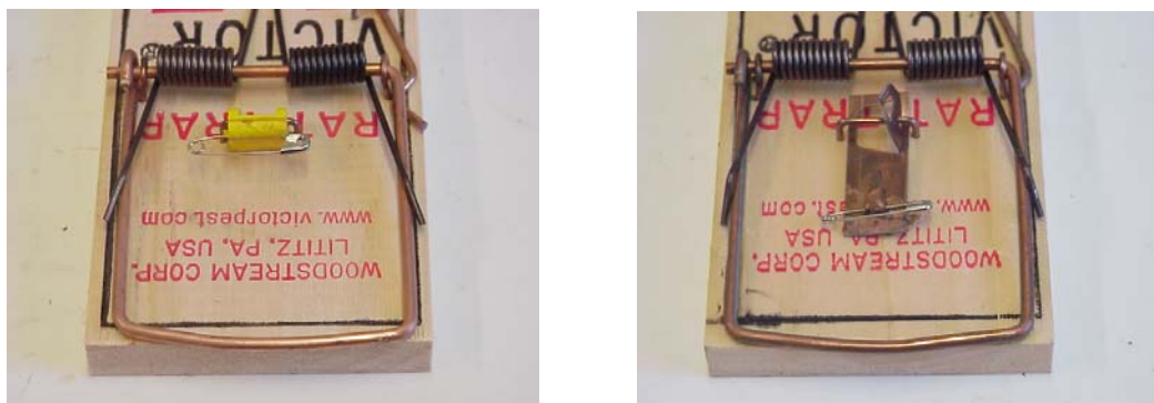
Fig. 1 Two types of Victor rat traps with modified triggers and safety pins attached for securing meat bait. Note the distance between the safety pin (bait) and striking bar is significantly less in the right-hand trap.
