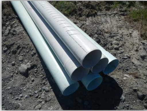
Figure 12: Gallery conduit with machine cut perforations
