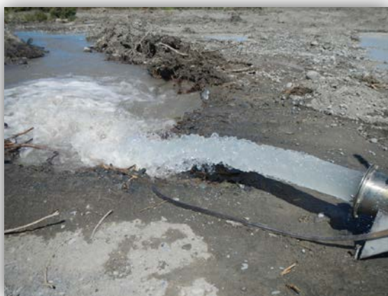
Figure 13: Discharge during a gallery test
