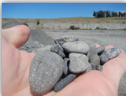
Figure 9: Washed infiltration pack material
