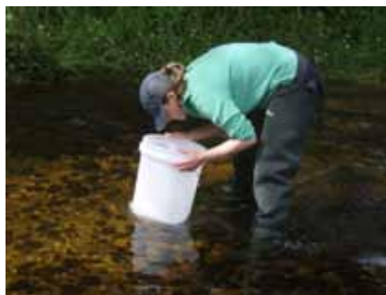
Figure 3: Operator estimating % cover of fine sediment of area visible through viewing box.
