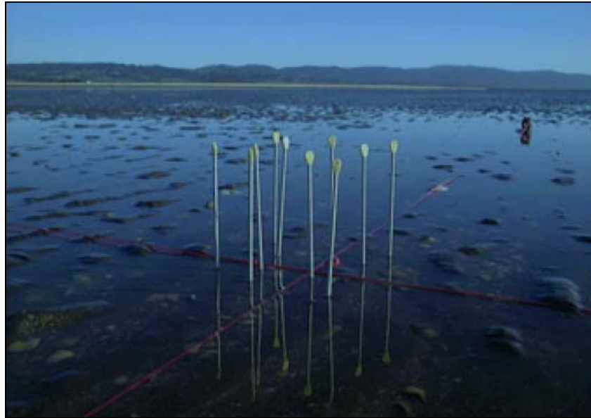
Figure 6. Measuring depth to the sediment plate using knitting needles. Several measurements are taken at once to ensure depth to plate is measured and not depth to an obstruction (from: Gibberd and Carter 2003 p11).
