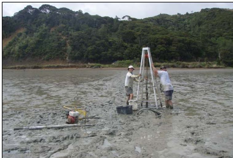
Figure 11. Vibracoring on an estuarine mud flat.
