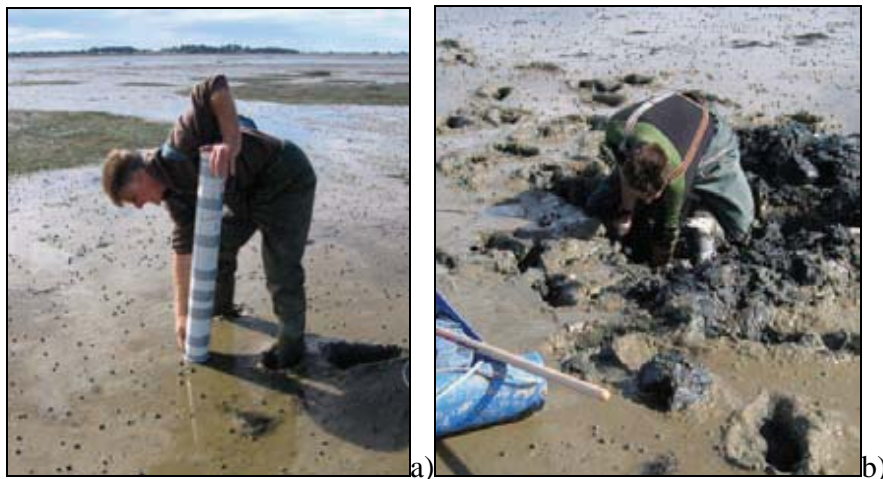
Figure 9. a) Inserting a sediment core by hand. b) Digging out the core for removal (from: Robertson and Stevens 2007a p9)
