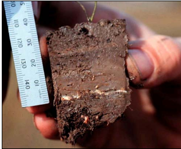
Figure 8. Example of measuring accretion using a marker horizon (from: USGS 2003)
