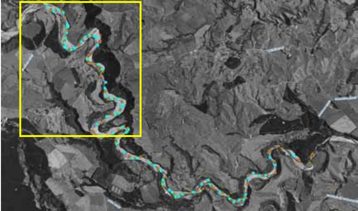
Figure 2: Tutaekuri River from Mangatutu confluence to Ngaroto Road. Blue dots indicate location of riffles. Yellow border indicates proposed survey reach.
