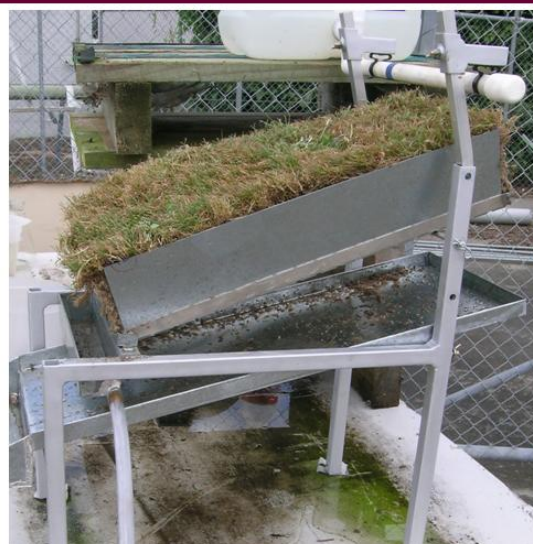
I. Applying water at set rate to the top of intact pasture slabs mounted to a certain slope (here 20%).
