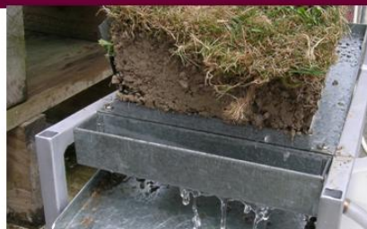
II. Measuring continuously and simultaneously surface runoff & leachate rates.
