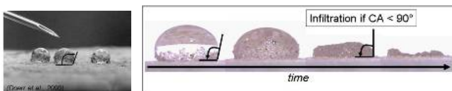
Figure 3.1.3. (a) The contact angle is a measure of the degree of soil water repellency (SWR). (b) The persistence of SWR is measured with the water drop penetration time test.
