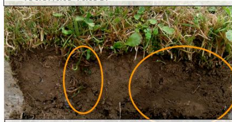
III. Slicing pasture slab and visualising wetted soil after set amount of rain.
