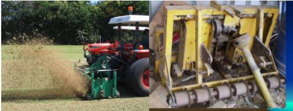
Figure 3.7.5. Dethatcher or scarifier (left) and Vibramole (right).
