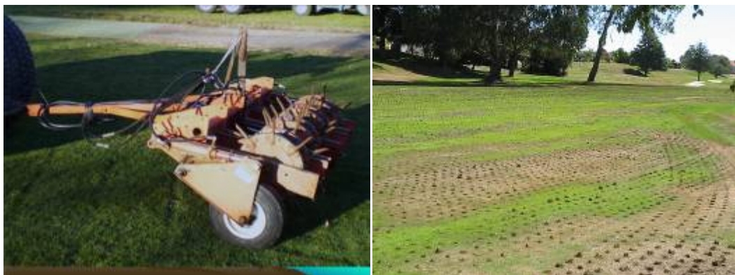
Figure 3.7.4. Tumble corer (left) for aeration and decompaction for soils of golf course fairways (right).
