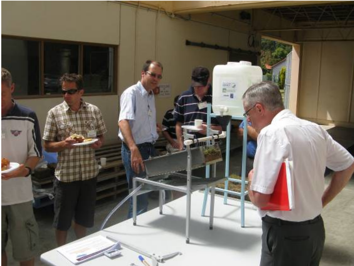
Figure 3.5.3. Markus Deurer (Production Footprints team, Plant and Food Research) explains the functions of the run-off apparatus. The apparatus can be used to measure the influence of soil hydrophobicity on run-off and overland flow.
