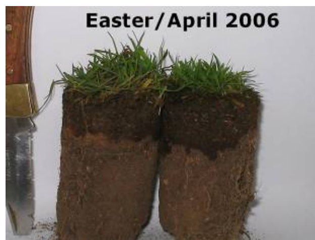
Figure 3.7.2. Low water infiltration and storage in hydrophobic soil cores taken from fairways of the Hamilton Golf Club after a heavy rain event (Easter 2006).
