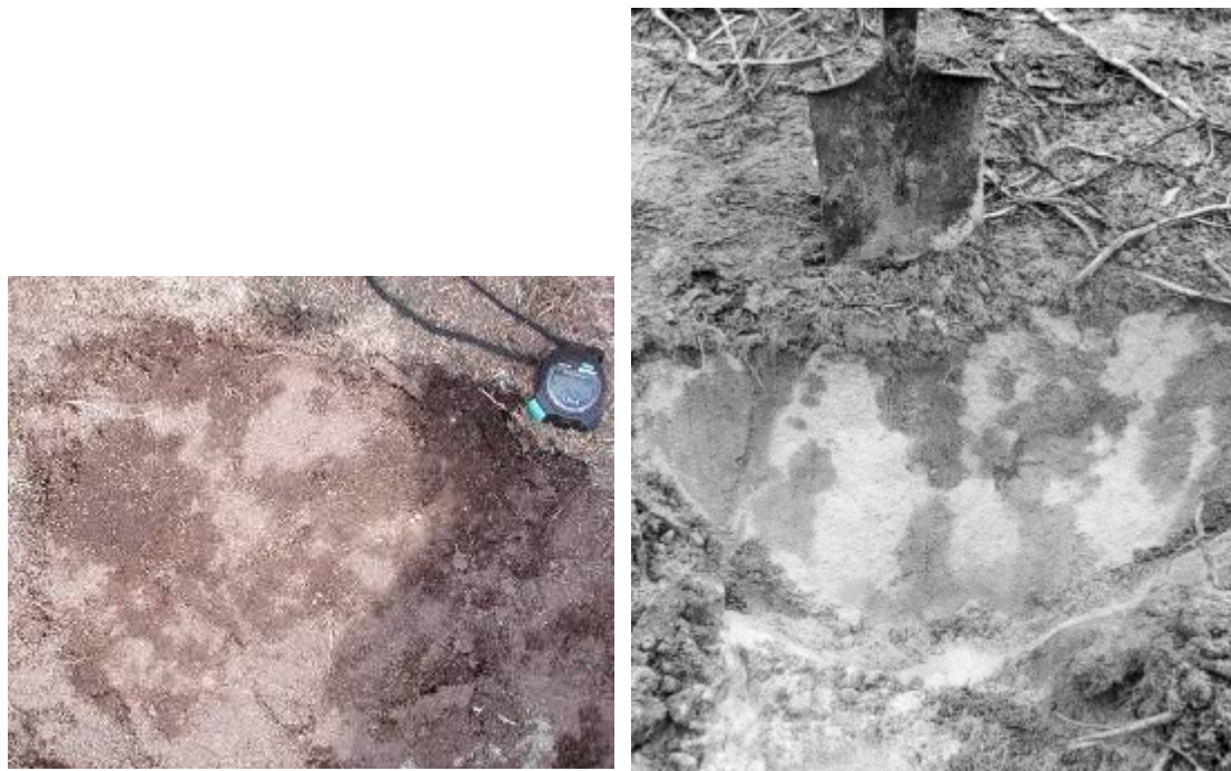
Figure 3.1.13. Uneven water storage in soil profiles with SWR. Left: Wetting pattern of the soil surface (view from the top) after a two-hour water infiltration experiment. Right: Wetting pattern after a large rainfall event (75 mm in 3-4 h). The photo was taken from (Doerr et al. 2000b).
