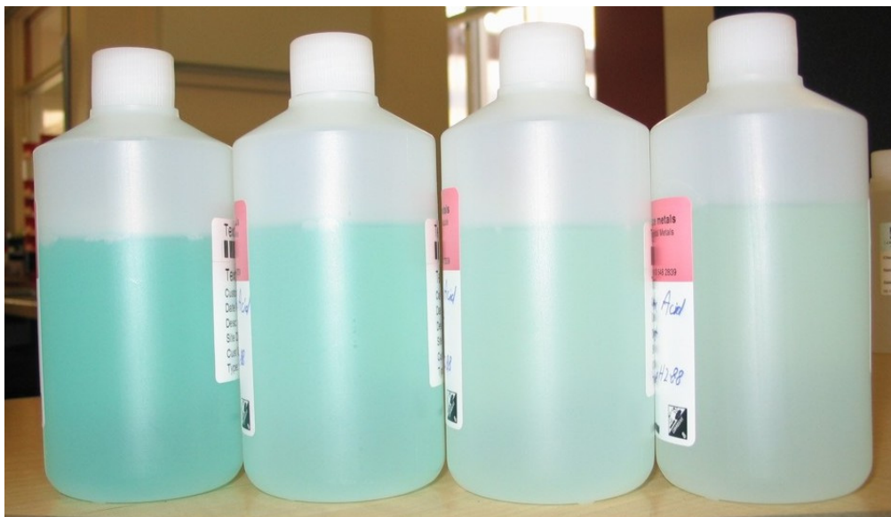
Figure 2. Filtered leachate from the block castings, showing colour gradation. Increasing cement addition from left to right (15%, 25%, 40%, 50%).
