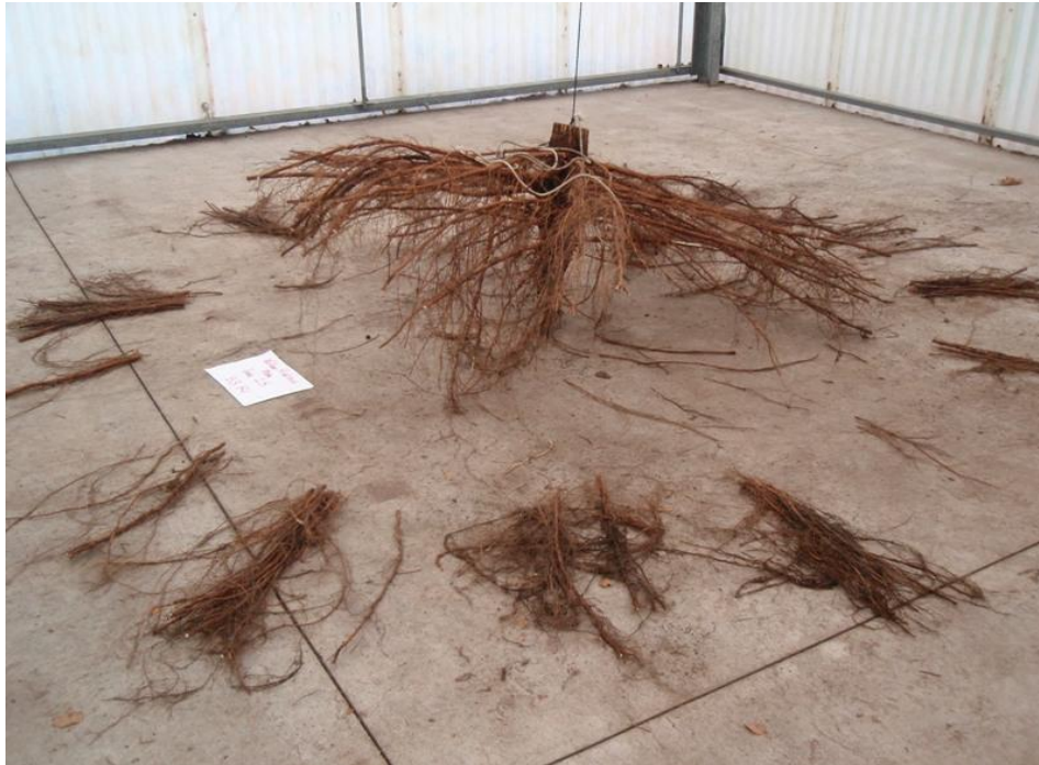
Figure 9 Partitioning of a 9-month-old willow root system from the Gisborne trial to measure the distribution of root length and biomass in 50-cm radial increments relative to the root bole starting from the outermost extent of the longest root. (Photo: Chris Phillips, Landcare Research).
