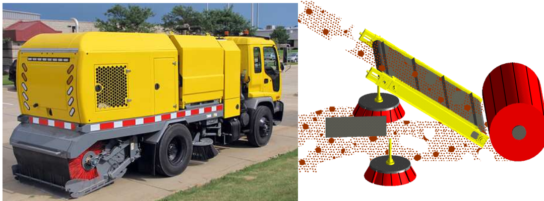
Figure 1: Left image, example of mechanical street sweeper (from Wayne Sweepers, LLC website, www.waynesweepers.com ); right, a schematic showing conveyor belt system for transferring the pavement sweepings into the hopper (from Elgin website www.elginsweeper.com ).
