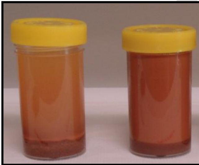
Figure 2. Clay dispersion in response to an exchangeable potassium percentage of 40% (left) or exchangeable sodium percentage of 40% (right).
