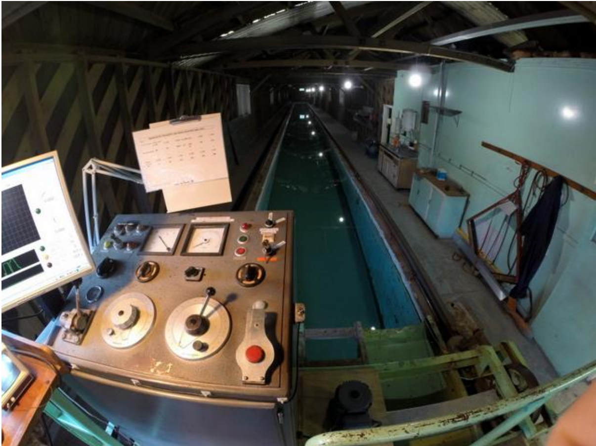
Figure 2 Right tool for the job – the velocity rating tank operated by NIWA Instrument Services at Kainga (Canterbury).
