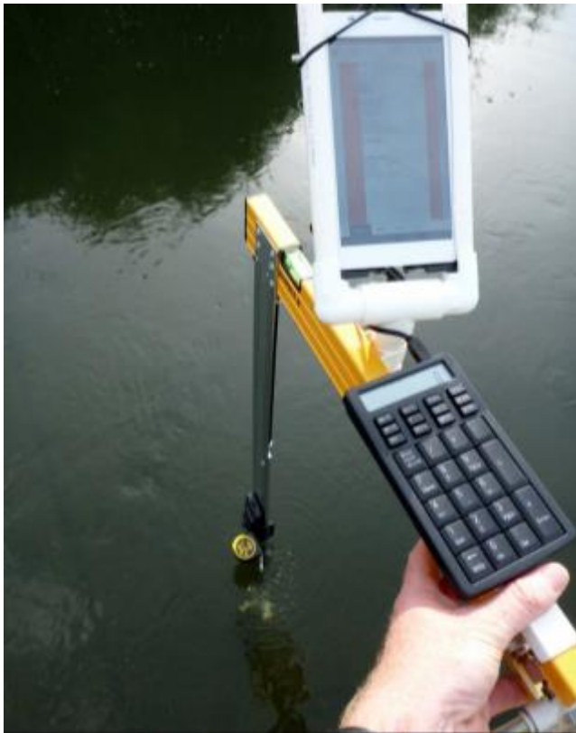
Figure 1 Rising-bubble method in action - the wading rod prototype for flow measurements.
