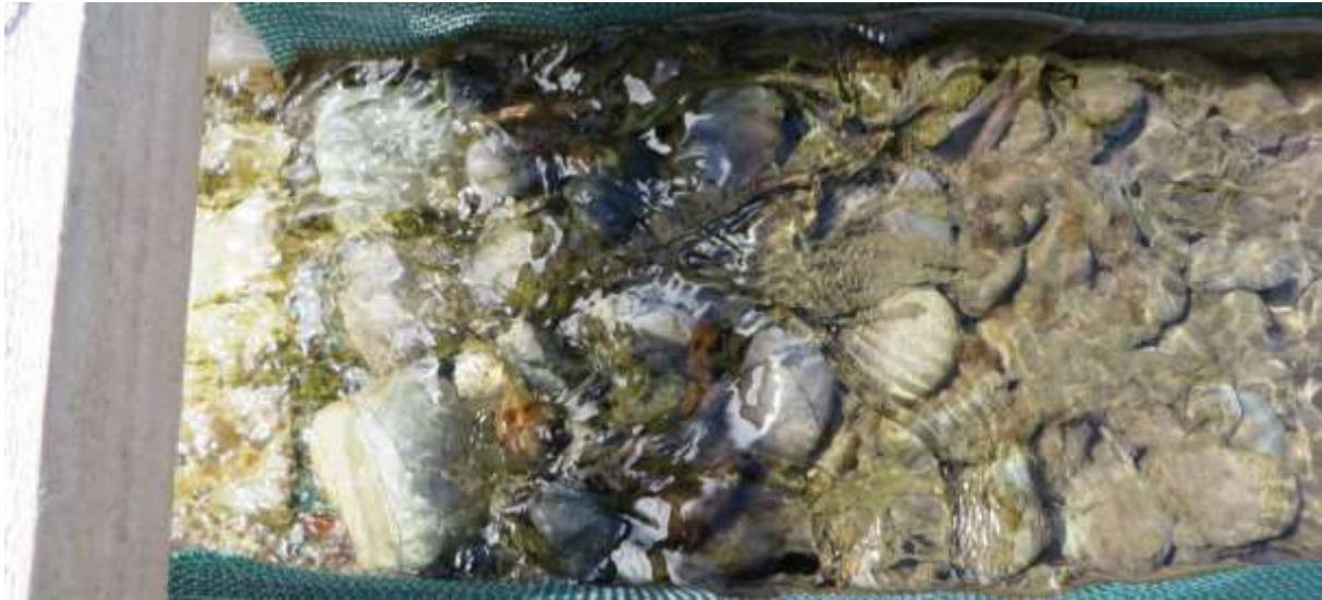
Figure 2-2: Invertebrate habitat at the downstream end of one of the channels on Day 24 of the experiment. Flow is from right to left. At the end of the experiment (Day 27), all the gravel was gathered into the mesh and invertebrates extracted from the entire sample in each channel.
