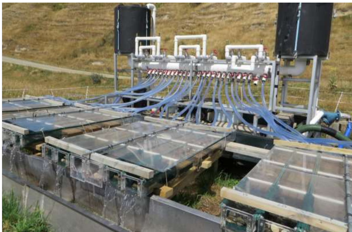
Figure 2-1: The flow-through experimental channel system located beside the Kowai stock-water race, Springfield, Canterbury. The system has 24 channels, but only 15 were used in this experiment to ensure that sufficient water was available for each channel to maintain near-bed flow velocities within the range typical in rivers and streams.
