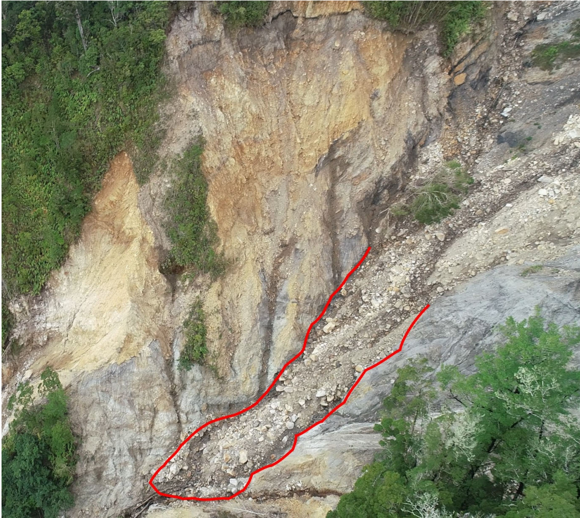
Figure 8. Debris supplied into the channel network from landsliding in the upper Lake Stream catchment (lobe of sediment in channel highlighted). Wetting and mobilisation of the material sitting in the bed of the channel is likely to be in the form of a debris flow or debris flood, given the steep nature of the channel bed at this point in the catchment and the apparent range of grain sizes in this material. The nature of sediment supplied to the Lake Stream channel from slope failure appears to include a range of crushed rock from the Kongahu Fault Zone, as well as boulders of more coherent sandstones from the Coal Measures. WCRC, supplied, dated 18 February 2021.
