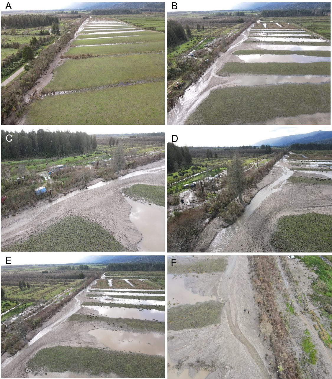
Figure 27. Sediment deposition in the Crows Nest channel alongside Crows Nest Road. (A) looking along the channel, (B) sediment splays into humped and hollowed paddocks, (C) channel vicinity of blocked culvert, which routed the current channel to the east (D), where it has deposited significant splays of sediment into humped and hollowed paddocks (C,D). (F) shows the contrasting channel dimensions between the former channel (narrow, straight, to the right of the photo, and the new channel, wide, sinuous, to the middle-left of the photo. Note the former channel does not have the capacity to transport the sediment and discharge now being routed along this course. WCRC supplied (photos obtained July 2022).
