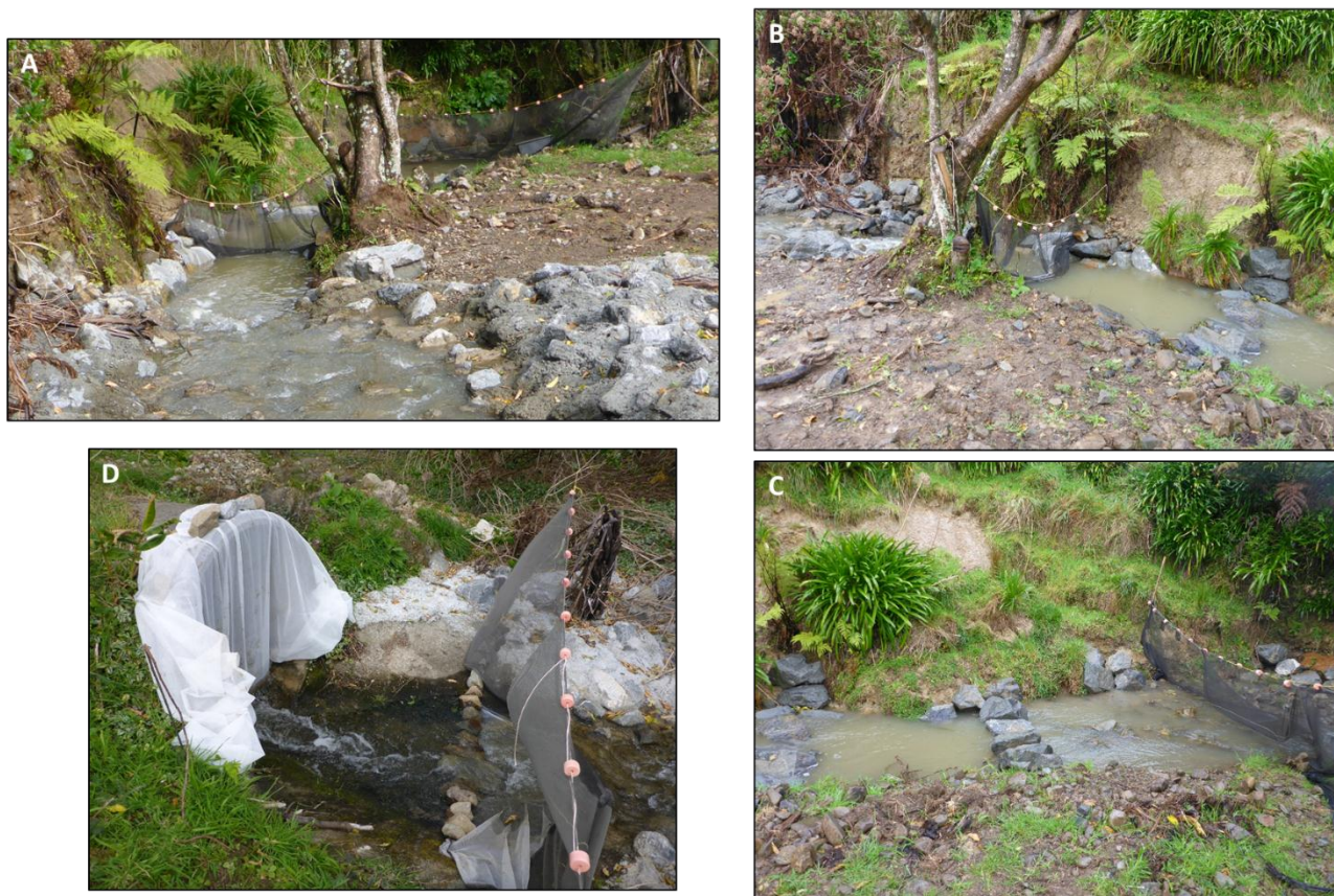
Figure 5-4: Downstream barricades installed in Kara Stream during the inanga passage trial. A - C Barrier nets deployed during the rock-ramp trial. D, Barrier nets deployed for testing inanga passage through the culvert independently of the rock-ramp.
