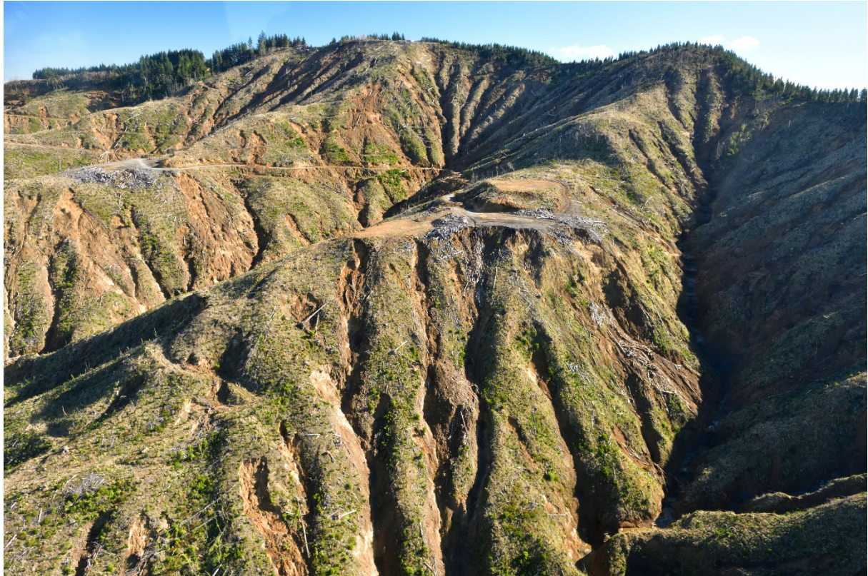
Figure 4.7 Shallow soil slides and debris flows with source areas in fill slopes below a landing on recently logged slopes in the headwaters of Takamapohia Stream, tributary of the Mangatokerau River (Te Mauranga Forest) (D. Townsend, GNS Science; 11 July 2018; D85_7836).
