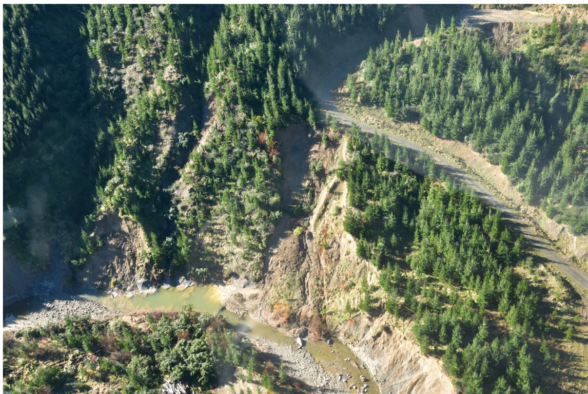
Figure 4.13 Debris slide directly coupled to the channel of the Mangaheia River, on Drysdale forestry road above Five Bridges. Sediment and woody debris have been delivered directly to the channel (D. Townsend, GNS Science; 11 July 2018; D85_8043).
