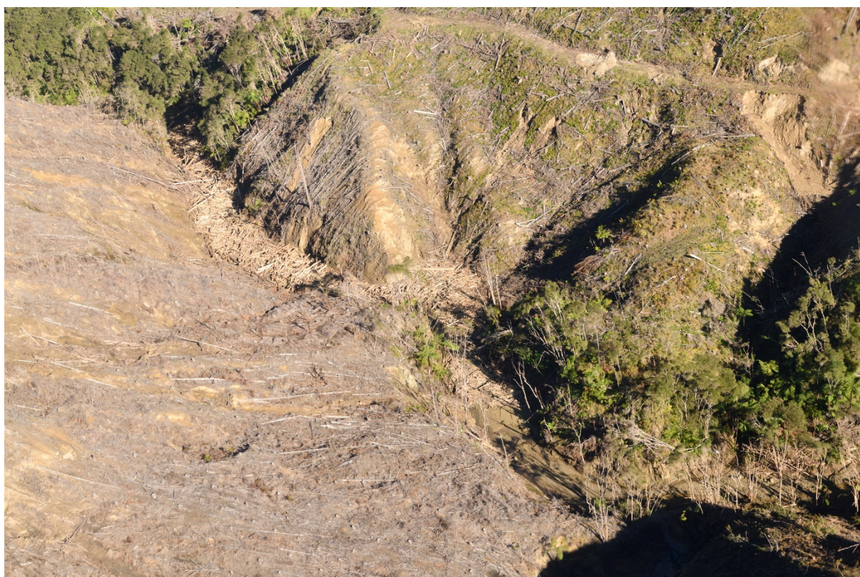
Figure 4.14 Woody debris generated from logging activities and transported by shallow soil slides, debris slides and debris flows stored in first order stream channels in the headwaters of Tapaue Stream, Paroa Forest, Uawa Catchment. (D. Townsend, GNS Science; 11 July 2018; D85_7894).
