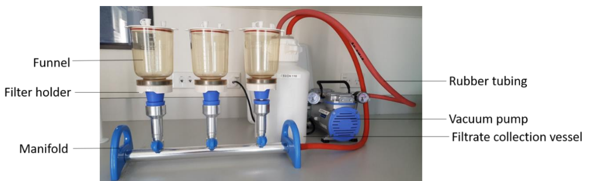
Fig. 1 - Filtering system for lab-based filtering of water samples. Three-fold manifold (magnetic system).
