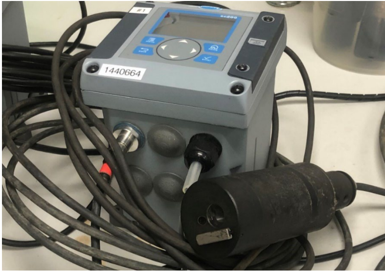
Figure 2-4: Hach Solitax sensor with controller unit. Note the brush wiper unit that wipes across the face of the sensor to keep the optical windows clean.
