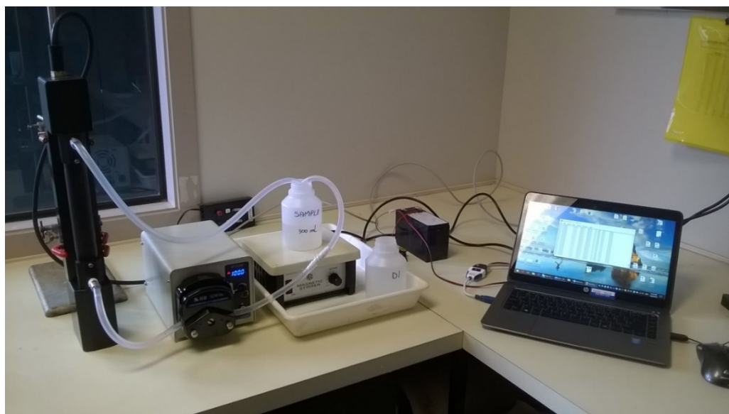
Figure 2-7: WET Labs® C-Star beam transmissometer set up in flow-through mode for laboratory measurements of beam attenuation coefficient (beam-c). L to R: C-Star sensor with flow-tube fitted (vertical mounting), peristaltic pump, diluted sample (stirred by magnetic stirrer), pure water storage flask, and laptop computer running Terra Term web 3.1). The C-Star emits a beam of green light (530 nm) and measures the fraction transmitted through the water sample.
