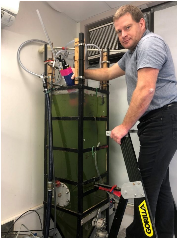
Figure 2-3: Mounting the EXO2 Sonde in the test tank. Three turbidity sensors were fitted to the same sonde body (blue cylinder). The sonde is taped (pink fluoro tape) to an aluminium rod for mounting the sensors (at the correct height and orientation) using retort clamps to fix the rod to a stage above the tank. The tank contained pond water (suspended phytoplanktonic algae) when the photograph was taken.
