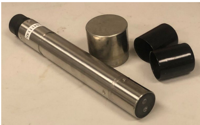
Figure 2-5: WTW VisoTurb turbidity sensor. (Storage endcaps removed).
