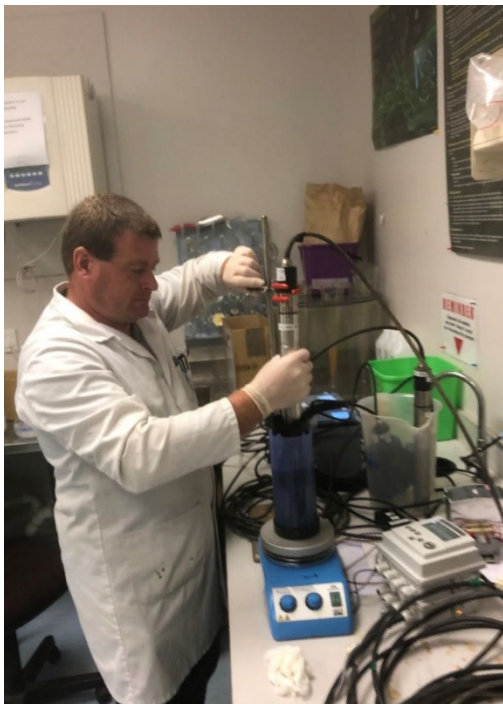
Figure 2-8: Calibration to formazin standards before measurements on natural suspensions. A WTW VisoTurb sensor is being calibrated, using the EXO2 sonde base as a beaker, and with magnetic stirring (blue stirrer unit). The WTW controller is the ivory-coloured box (with readout) to the right of the magnetic stirrer.
