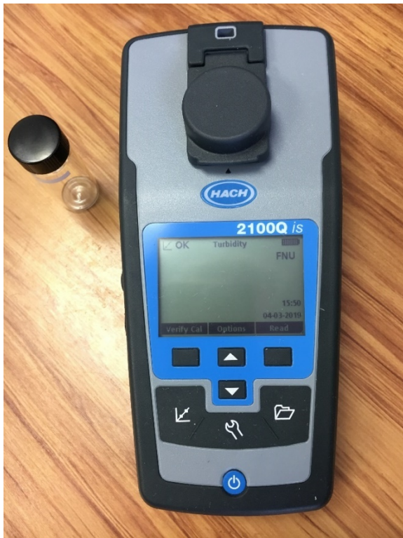
Figure 2-2: Hach 2100Q-is portable cuvette turbidimeter. One of the cylindrical cuvettes (with black screw top) used to contain water samples is shown to the left of the instrument.
