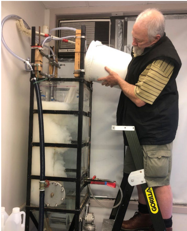
Figure 2-11: Adding kaolinite to the test tank. The tank was partly filled with degassed tap water, and after addition of the kaolinite slurry the tank volume was topped up to the operating level (red line, 163.3 L).
