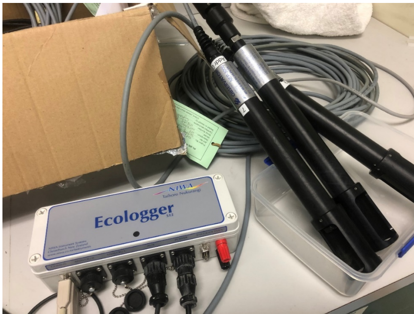
Figure 2-6: Observer Analite NEP 5000 turbidity sensors. A housing (shroud on bottom right) protects the optical face of this sensor with its small rotary brush unit. The three sensors were connected to the NIWA Ecologger (shown) outputting to a laptop computer running Starlog V4.
