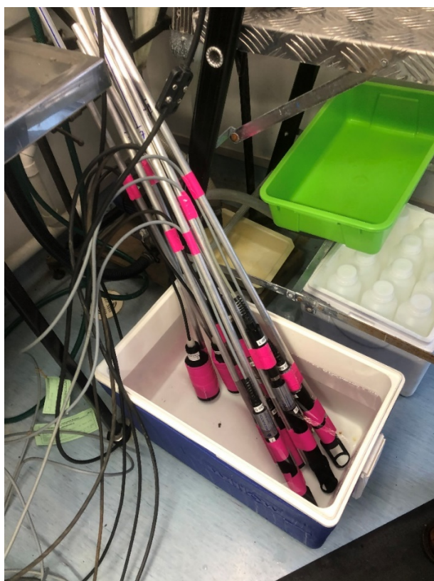
Figure 2-15: Storage of field turbidimeters in a chilly bin of tap water between test-tank deployments.
