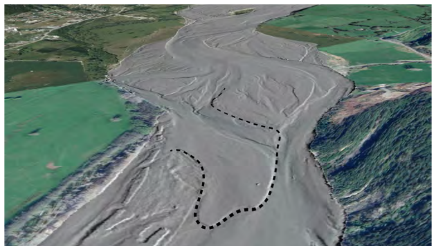
Figure 2-22 Recent emplacement of a gravel lobe upstream of the Walker Rd gravel extraction site, sourced mainly from erosion at a bend 200 m upstream. Viewpoint is looking upstream; extraction site is at lower left. The hillshade model comes from a photogrammetric survey in Feb 2020 (cf. Section 3.2).
