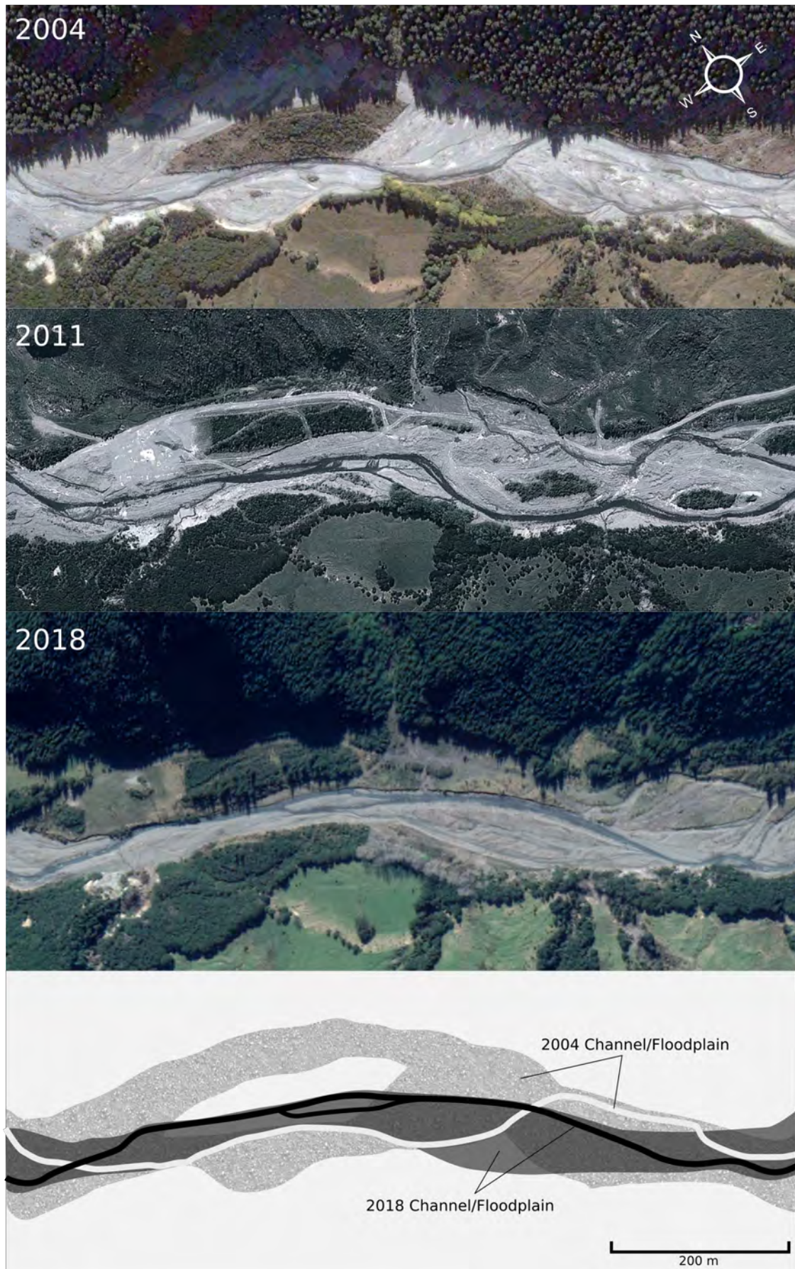
Figure 2-10 Aorangiwi River, upstream of the Matahaia Bridge (see Figure 2-9). Flow is left to right. Gravel operations were carried out in-stream, gravel was stockpiled on the river bed, and note the absence of barriers between flowing water and active excavation. The example emphasizes the capacity for relatively rapid change in sediment supply, even following cessation of gravel extraction (©Digital Globe, Google Earth).
