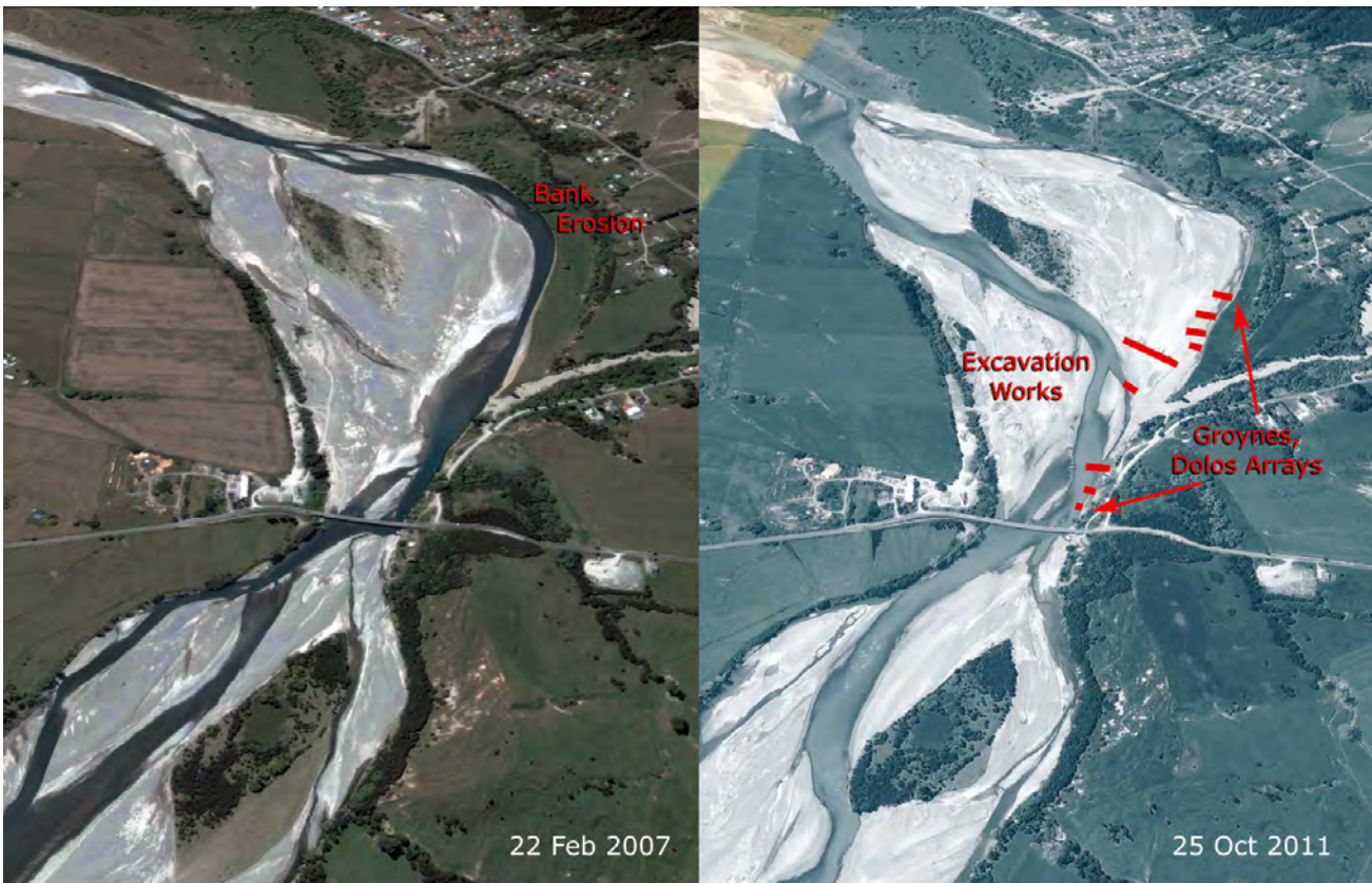
Figure 2-25 The realignment of the Waiapu River was carried out through a combination of gravel extraction on the left bank and emplacement of dolos structure as groynes on the right bank. This combination of strategies has successfully moved the river over to the left bank. Deposition around the groynes has ensured that the channel is not likely to avulse back toward the right bank.
