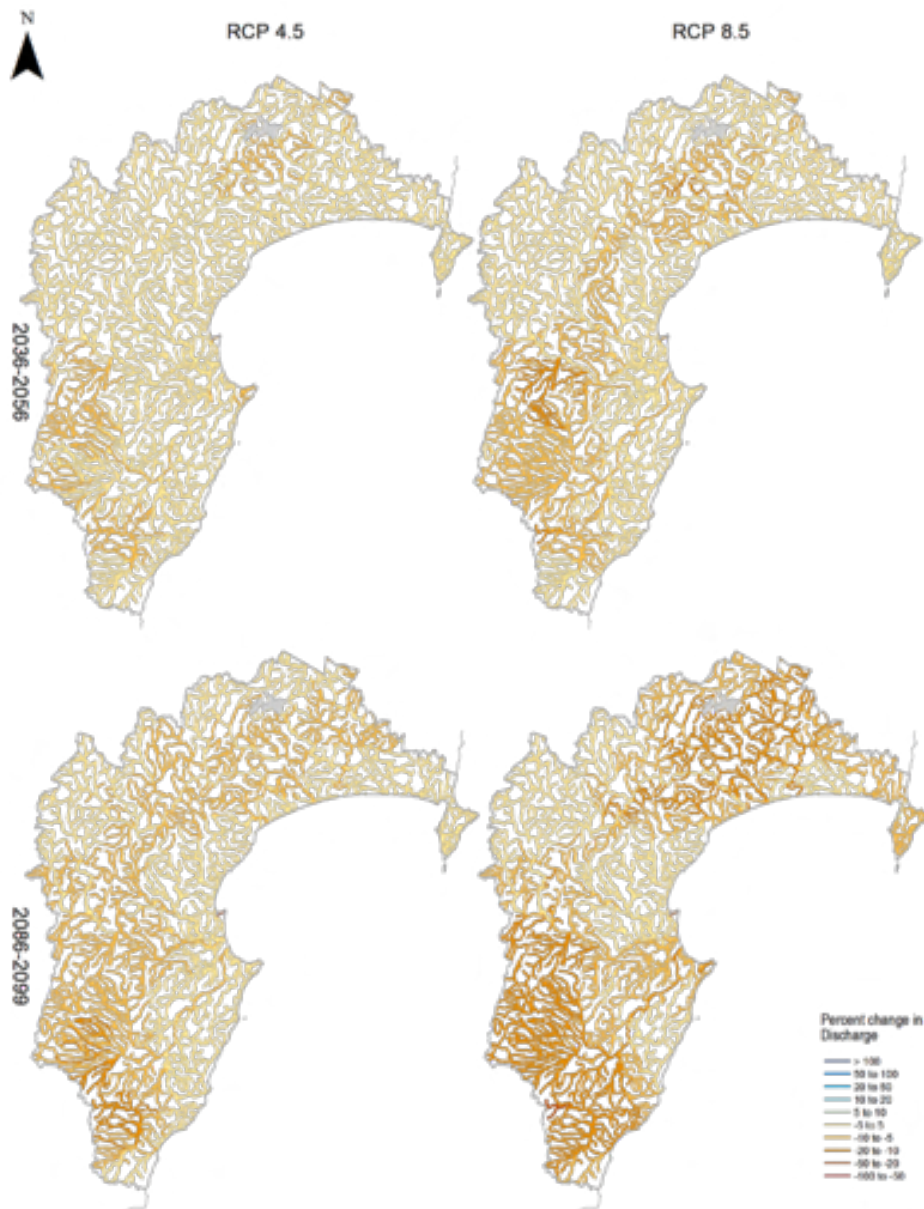
Figure 7-2: Percent changes in multi-model median of the mean discharge across Hawke’s Bay region for mid (top) and late-century (bottom). Climate change scenarios: RCP4.5 (left panels) and RCP8.5 (right panels). Time periods: mid-century (2036-2056) and end-century (2086-2099).
