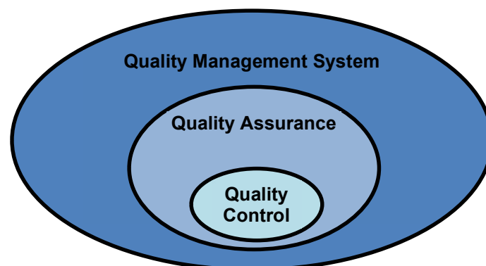
Figure 3-1: Relationship between a quality system, quality assurance (QA) and quality control (QC). QA and QC requirements are defined during the monitoring design process when monitoring objectives are established.
