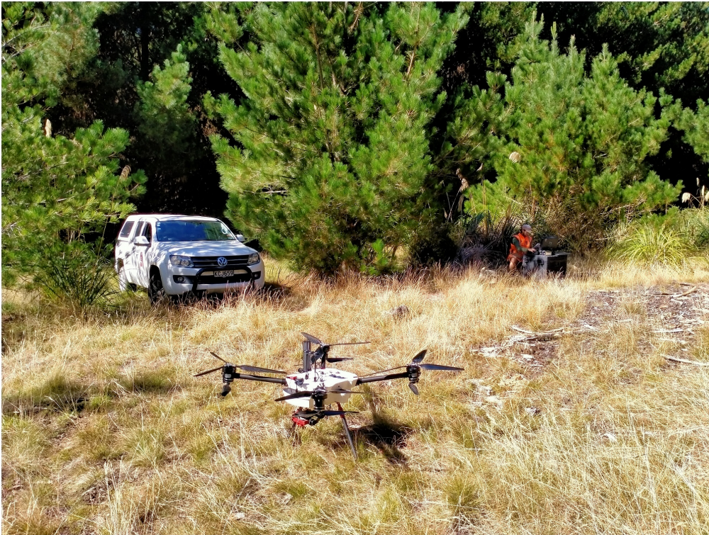
Figure A1.1 Altus LRX UAV with multispectral camera attached (see Figure A1.2 below).
