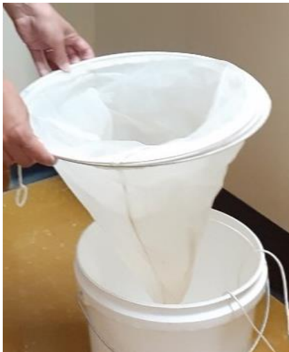
Figure 3: Modified nets (350, 250, 65 \mu\text{M} ) used for collection of stygofauna. Nets are stacked and used to filter pumped well water.
