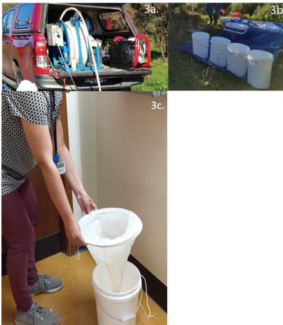
Figure 3: Sieve sampling images. Figure 3a shows the Bennett pump; Figure 3b indicates a suggested 100 L sampling layout (note 20 L buckets were used in this case); Figure 3c shows the sieve set up with the 250 \mu\text{m} net on top of 150 \mu\text{m} , on top of 63 \mu\text{m} net.
