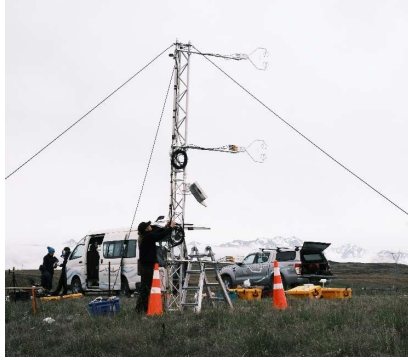
Figure 6-3: Left: Wind tower with three Campbell Scientific CSAT3B sonic anemometers. Centre: Vaisala WXT536 climate station. Right: ProTech QM1646 handheld anemometer.
