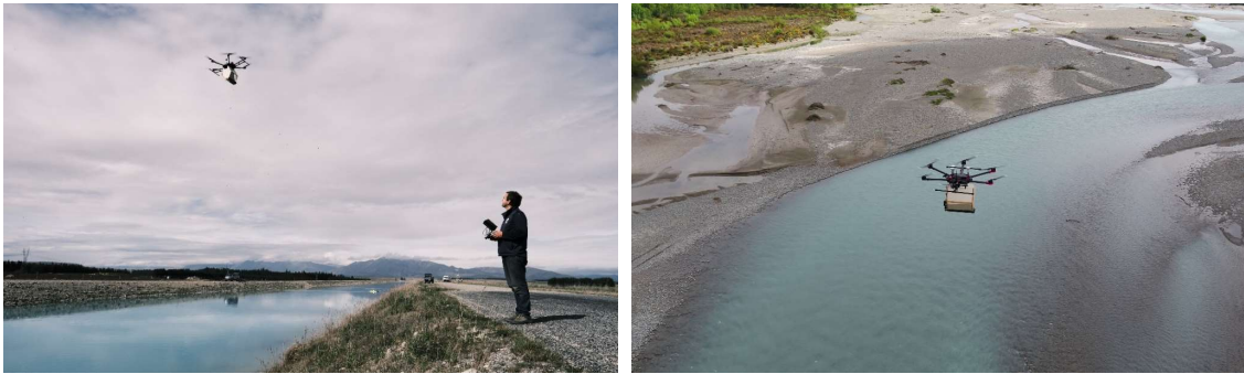
Figure 7-1: NIWA environmental monitoring technician Hamish Sutton flying a tracer particle distribution system in the Tekapo Canal (left) and Rangitata River (right).
