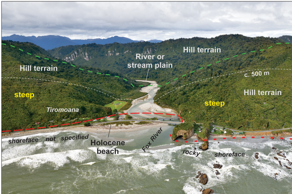
Figure 4.10 Overview of coastal environment at Fox River mouth, between Westport and Greymouth. See Figure 4.7 for explanation of symbols and terms. Photo D. Townsend, July 2021. VML ID: 259915.
