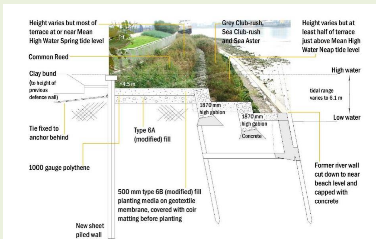
Figure 3-6: Vertical sheet wall replacement with gabion terraces at Greenwich Peninsula Terraces North West. (source: https://www.estuaryedges.co.uk/case-studies/greenwich-peninsula-terraces-north-west/ )
