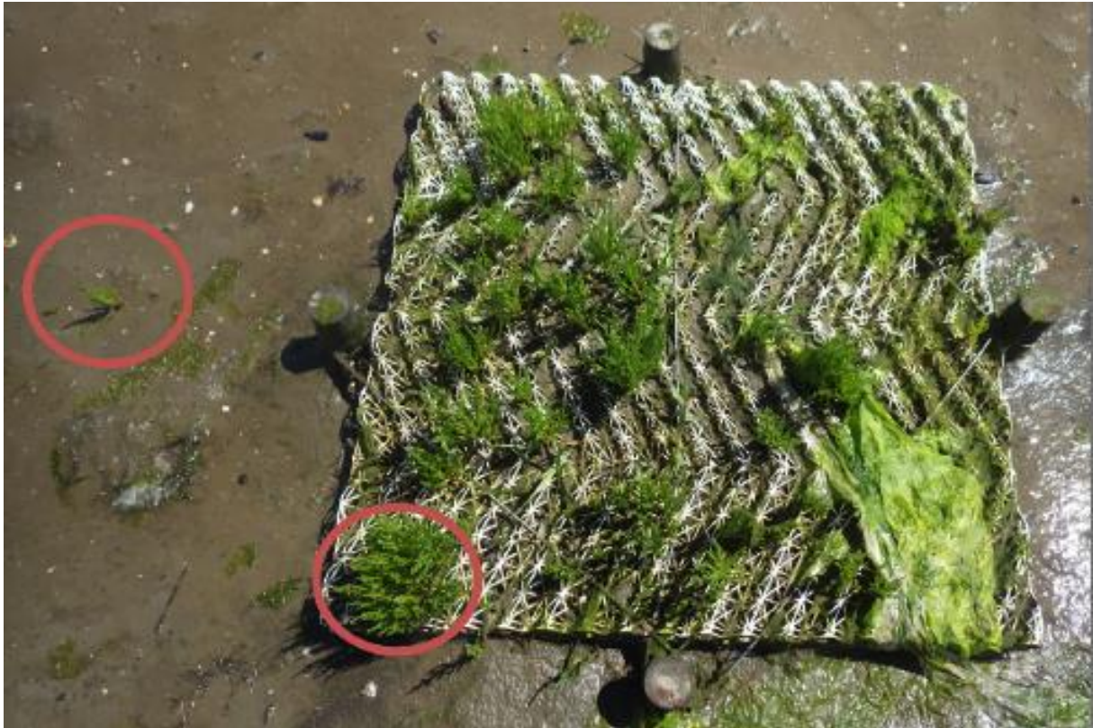
Figure 3-3: Artificial structure used in the field experiment at Texel in the Netherlands. The structure supported high densities of salt-marsh recruits, predominantly Salicornia sp., and recruits were considerably larger than those found in the nearby unmodified mudflat (source: Fivash et al. 2021).
