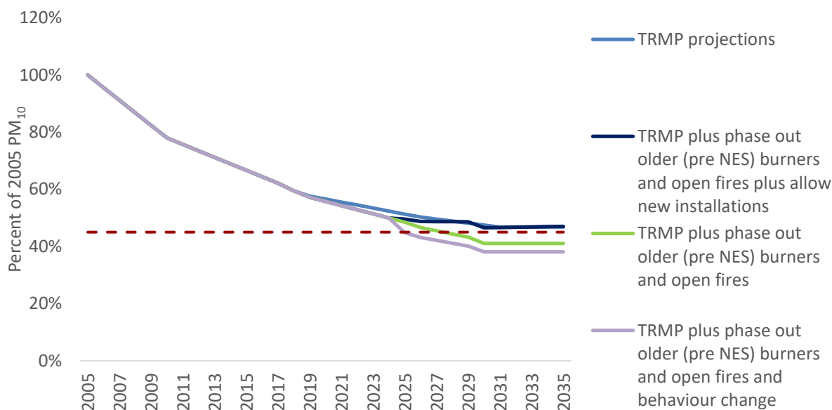
Figure 3-2: Phase out open fires and older burners not meeting the NES design standard for wood burners, with and without behaviour change to improve burner operation
