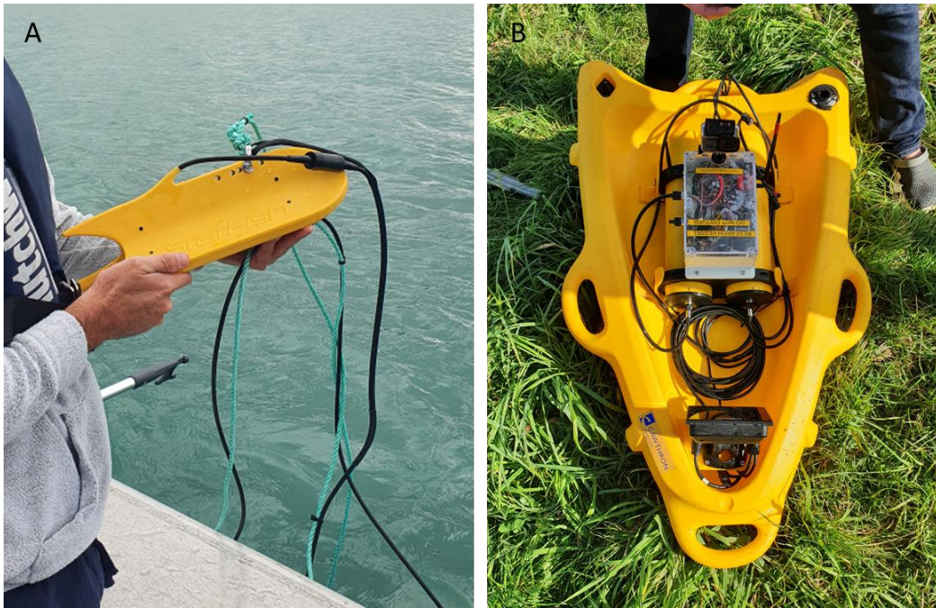
Figure 4. A) The towable sidescan system 'Blueprint Subsea StarFish' and B) the autonomous sidescan system.
