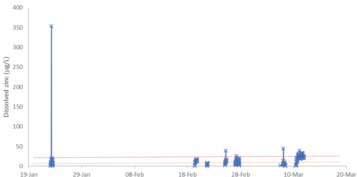
Figure 2-5: Dissolved zinc concentrations measured in an Auckland stream during different rainfall events. Orange line indicates acute GV (24 µg/L, from CCME (2018)) and orange indicates chronic draft DGV at index condition (4.1 µg/L). Zinc concentrations regularly exceed both acute and chronic GVs in this stream. Data collected 2004 from Auckland City Council study 78 .
