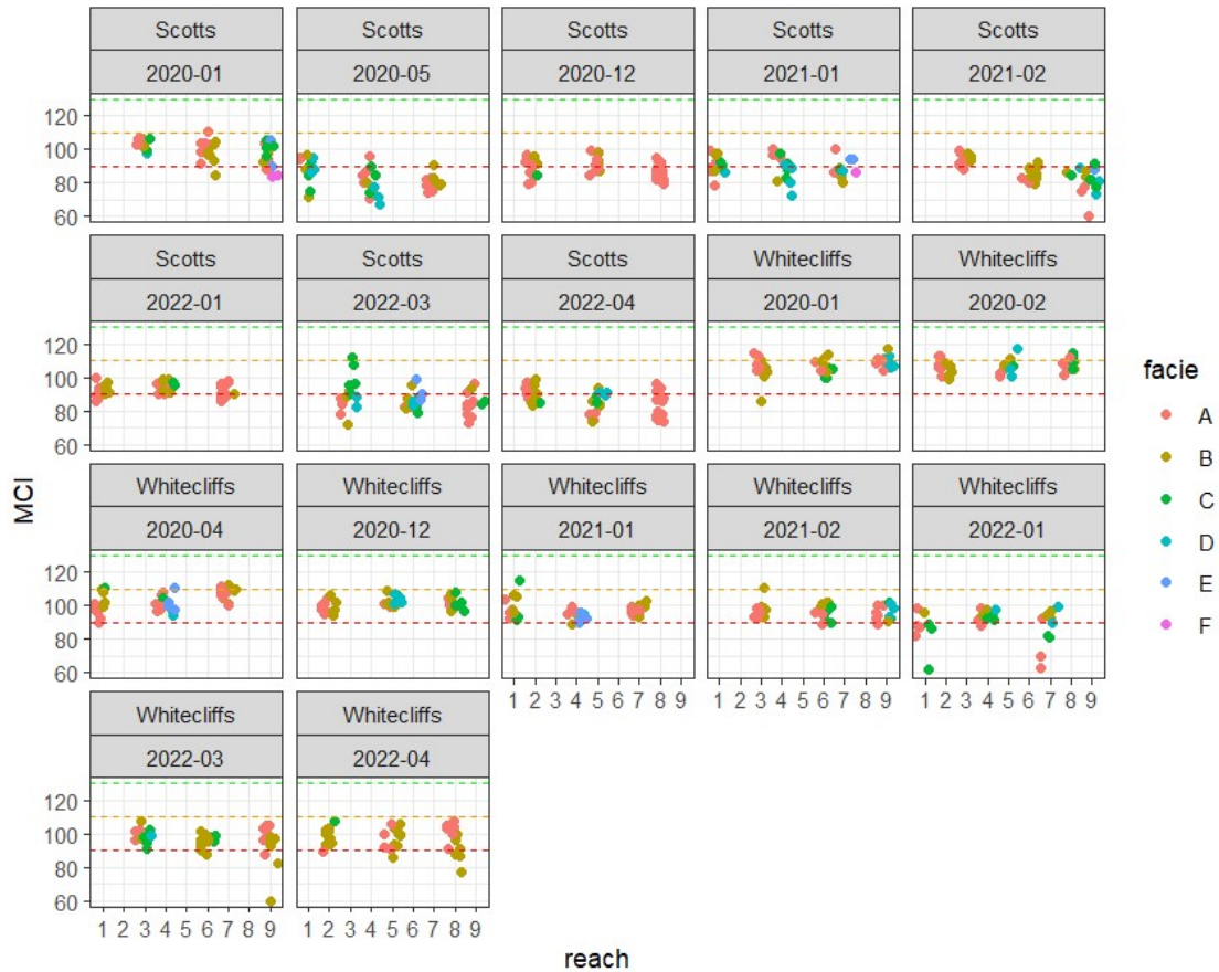
Figure 7-5: MCI values calculated for 13 Surber samples collected within three reaches (of nine permanently marked) at two sites on the Selywn River (Scotts Road and Whitecliffs) over multiple visits between 2020 and 2022. Facies are visually identified and mapped for each reach on each visit based on the substrate composition, water depth and velocity. Red, orange and green dashed lines indicate the NPS-FM attribute band thresholds for C/D, B/C and A/B, respectively.
