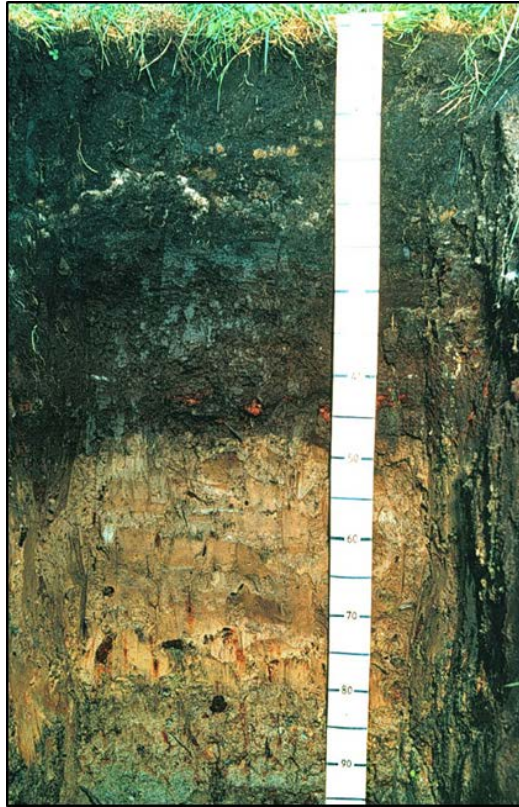
Figure 18. Peat soils have at least 30 cm of material within the top 60 cm that contain 18% of more C.
