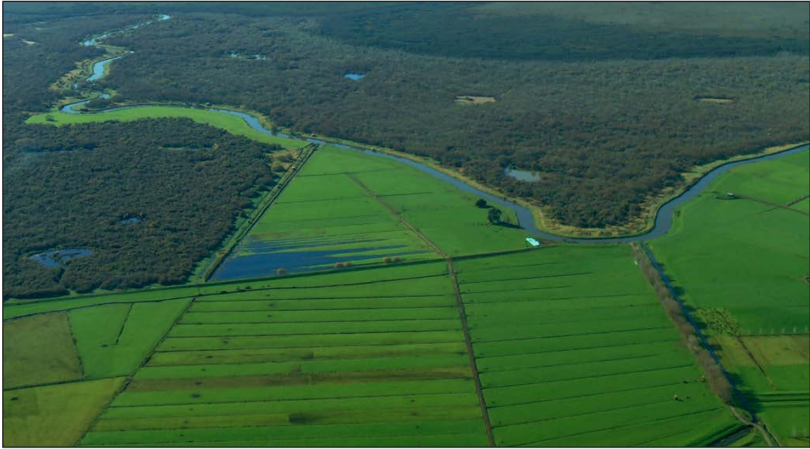
Figure 7. Even though an area is drained it may still be wet because there is little fall and the water table remains high.
