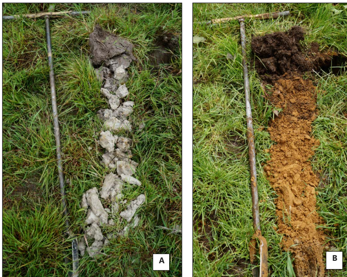
Figure 10. The dramatic difference in subsoil colour between a poorly drained soil (A) and a well-drained soil (B).
