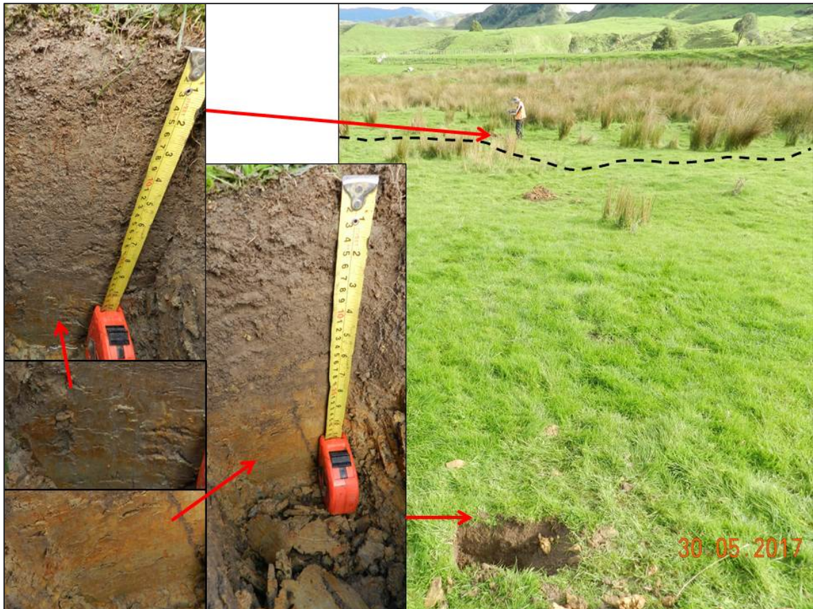
Figure 26. Changes in vegetation correspond to changes from mottled to gley profile form.
