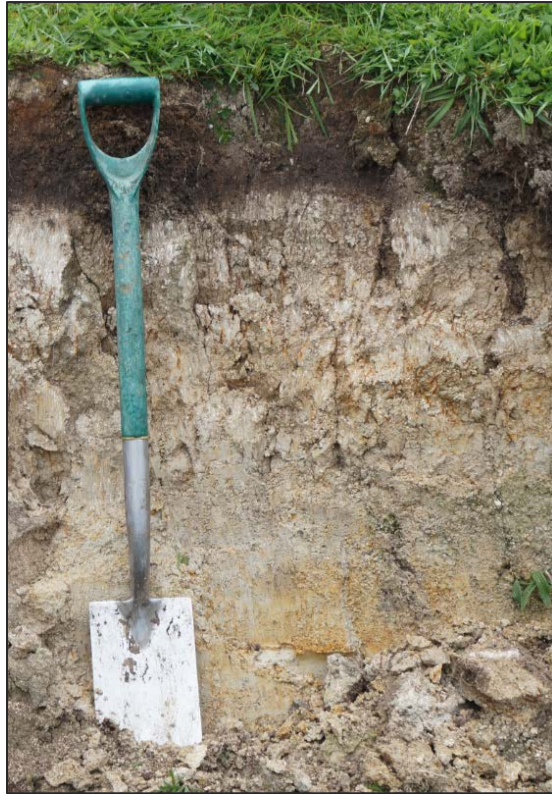
Figure 17. Low chroma colours and redox mottles typical of a gley profile form.
