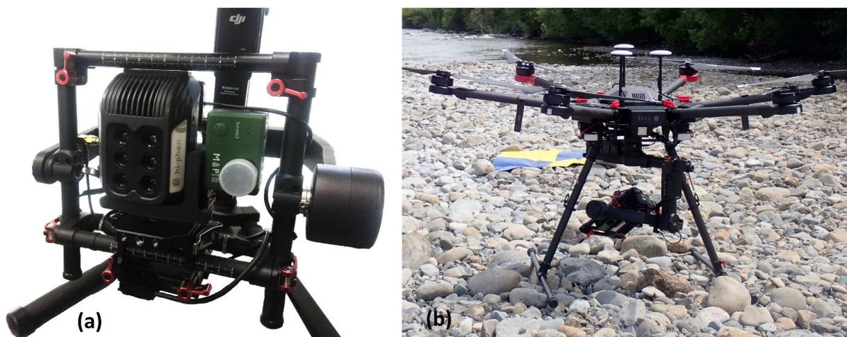
**Figure 3-5: (a) Mapir survey 3W and Airphen multispectral cameras mounted on a DJI Ronin MX Gimbal. (b) Ronin MX Gimbal and multispectral cameras deployed on a DJI M600 drone in the Hutt River.**
