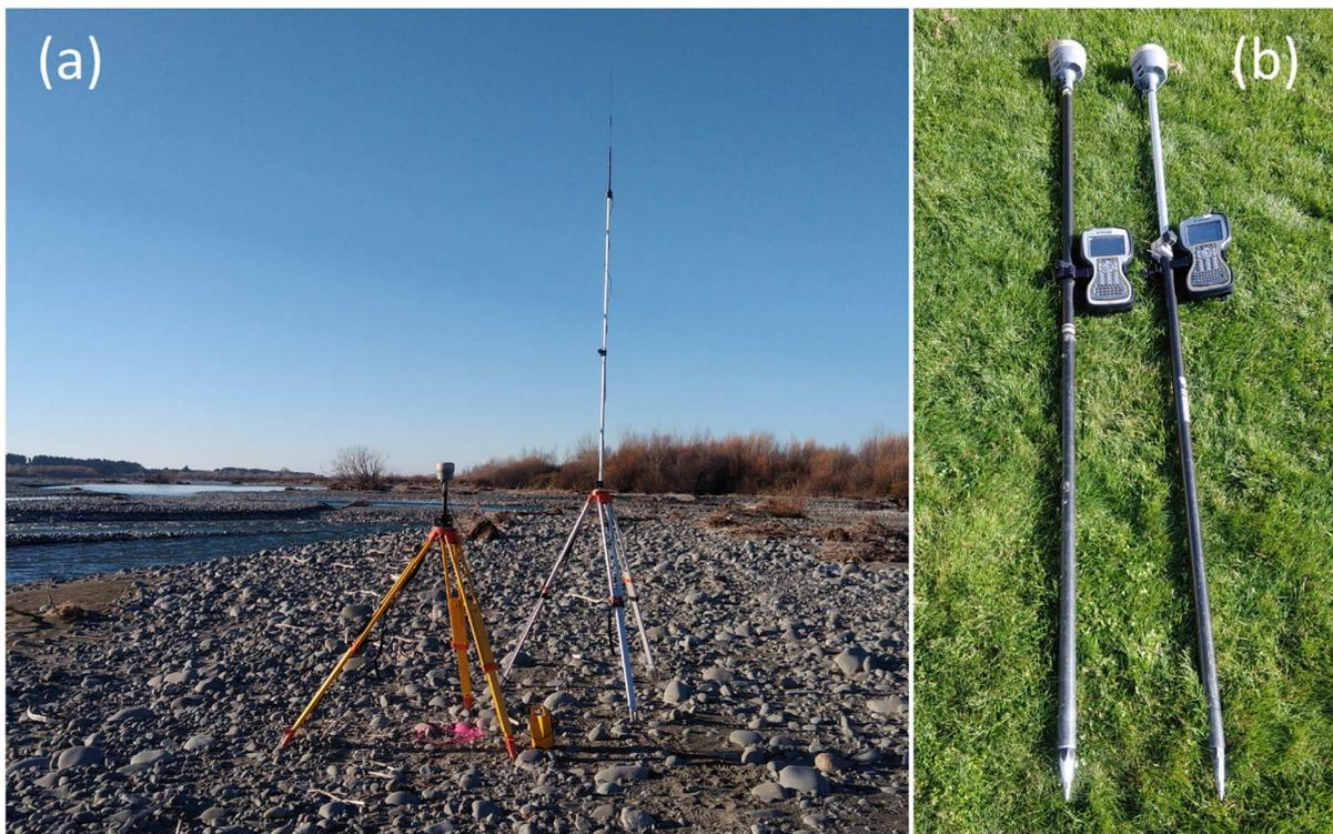
**Figure 3-8:** (a) Trimble R10 RTK GPS base station, (b) 2x Trimble R10 Rovers.
