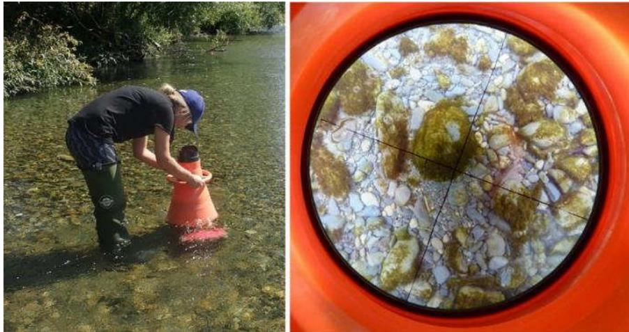
**Figure 5-1: A bathyscope is used to view the riverbed in wadeable rivers.**
