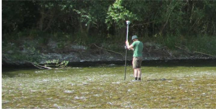
**Figure 5-4:** Surveyor performs RTK GPS ground truth measurements of cover classes throughout the study reach, then measures the locations of labelled markers (where biomass samples were taken).
