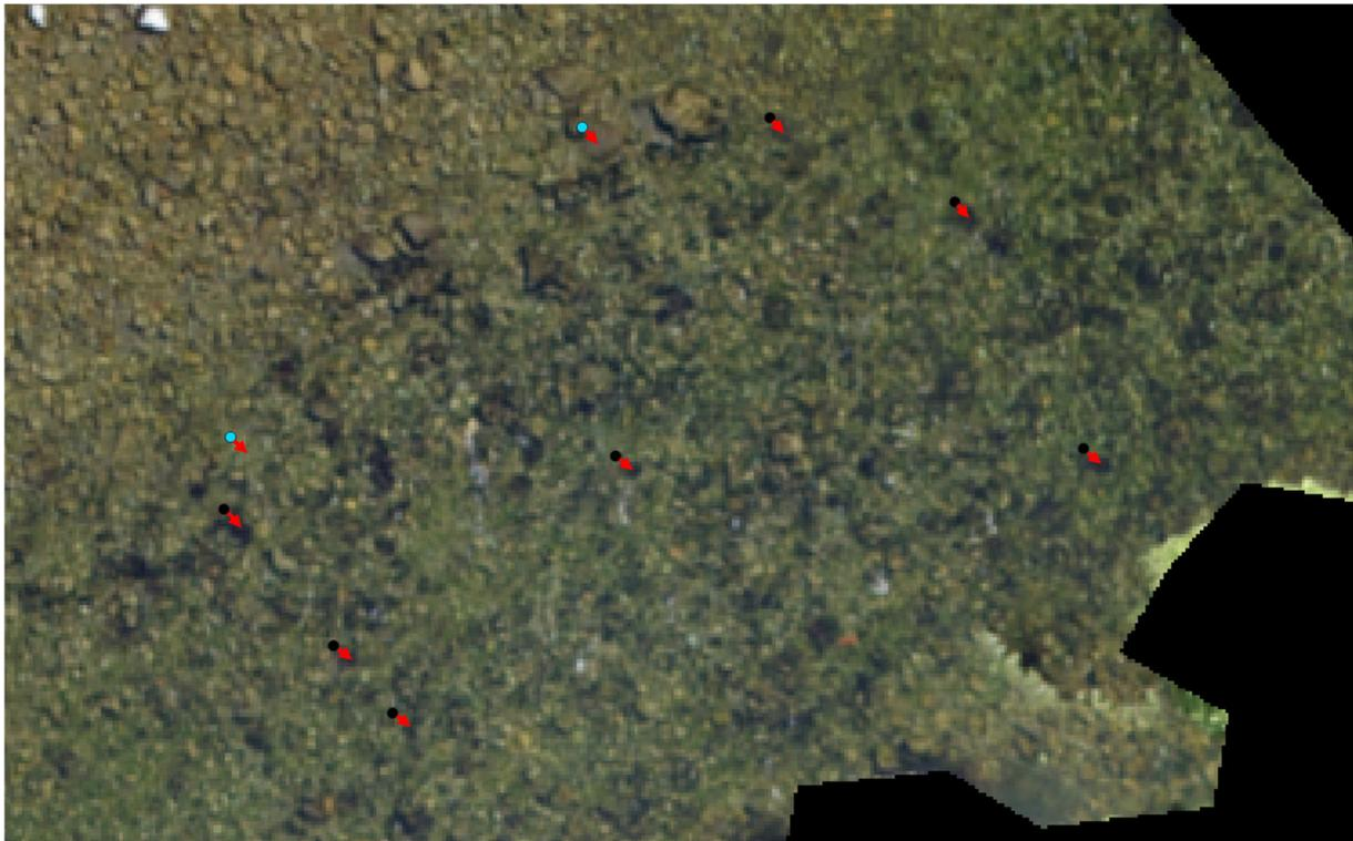
**Figure 7-12: Example of spatial discrepancies between objects apparent coordinates in georeferenced orthomosaics and their actual coordinates from RTK GPS ground truth surveys.**
