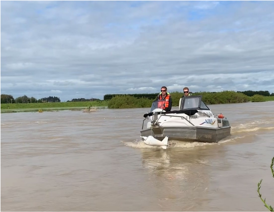
Figure 2-2: Example of depth-integrated physical sampling in Oreti River . using a depth-integrated D77 sampler, which provides the direct measure of representative suspended sediment concentration in a river.
