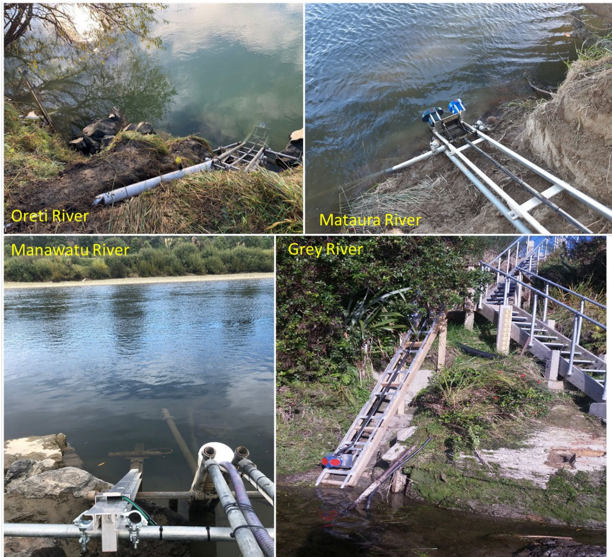
Figure 2-1: Side-looking acoustic backscatter profilers deployed at the monitoring sites. Teledyne ChannelMaster was used at the Oreti, Mataura and Grey Rivers. OTT-SLD was used at the Manawatu River.
