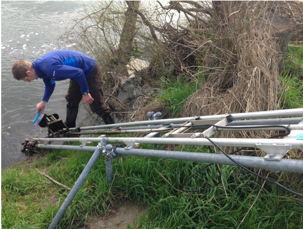
Figure 5-6: A sliding rail mount at Matura River and cleaning the sensor by Andrew Willsman (NIWA-Dunedin).
