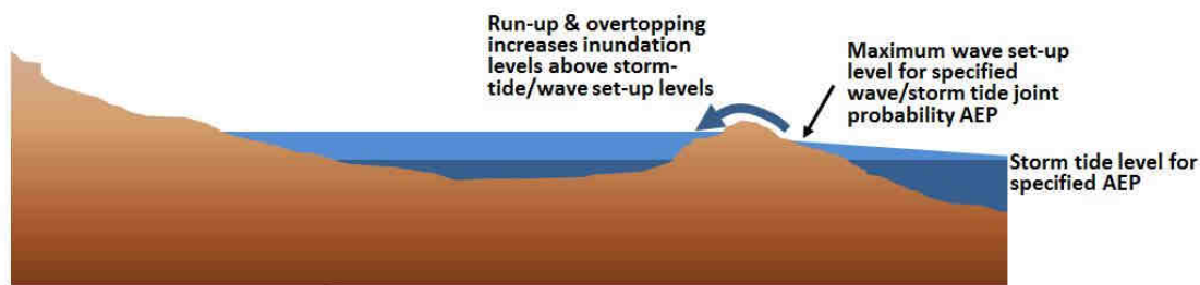
Figure 14 Overtopping of a coastal berm resulting in inundation levels that are greater than seaward storm tide or wave set-up levels.
