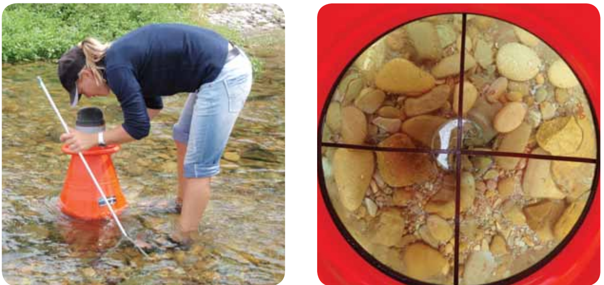
Figure 4-2. Photos of an underwater viewer used to assess fine sediment cover.
