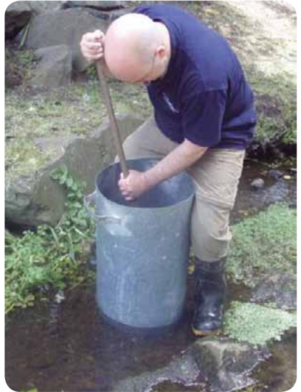
Figure 4-18. Large corers successfully applied to extend the physical limitations of the Quorer method.
