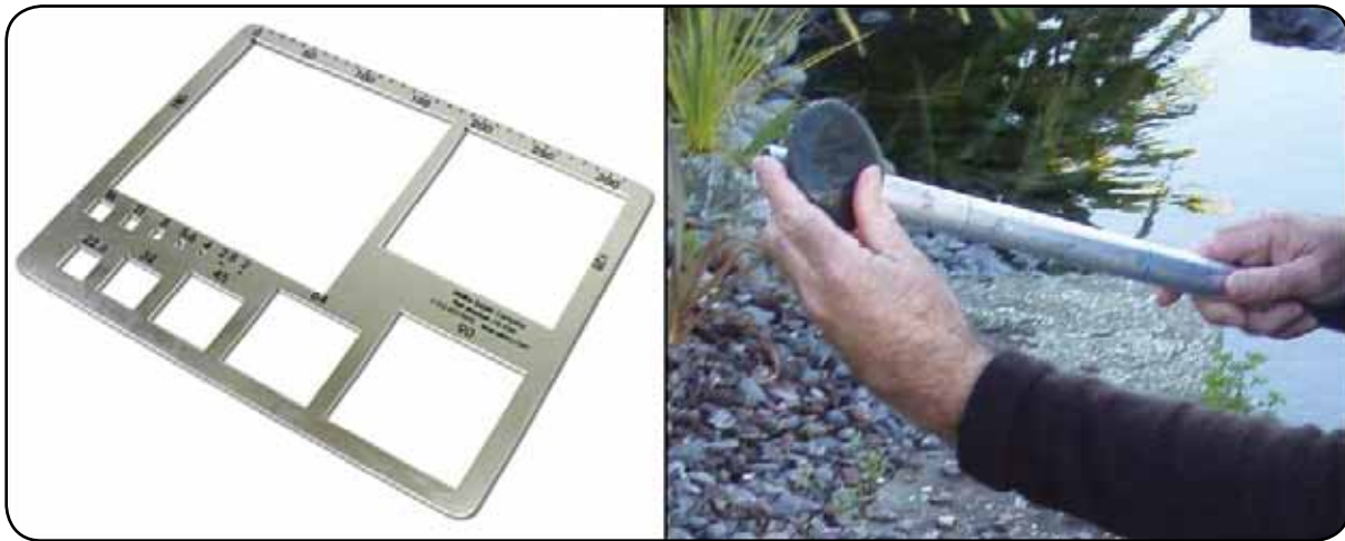
Figure 4-3. Photos of common tools used to measure particle grain size: a gravelometer (left) and a rod graduated with Wentworth scale size classes (right).
