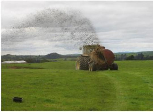
Photos 4 & 5: Side-delivery spreading system used for spraying flats and steep sidings.
