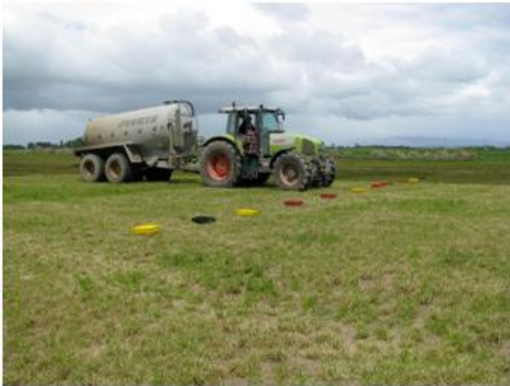
Photo 36: Slurry spreading pattern being measured.
