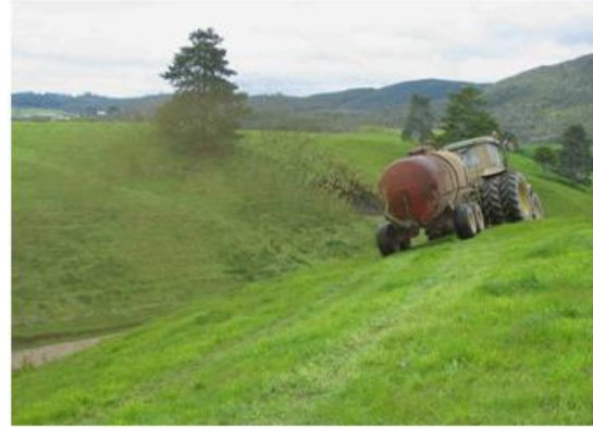
Photos 4 & 5: Side-delivery spreading system used for spraying flats and steep sidings.
