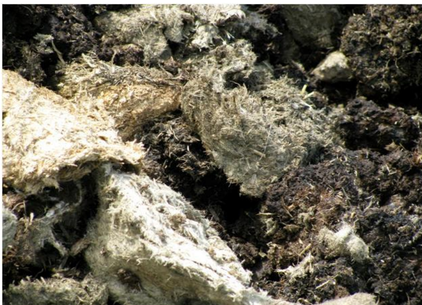
Photo 42: Solid fraction remaining after going through mechanical screw press separator (fresh and old solids visible).
