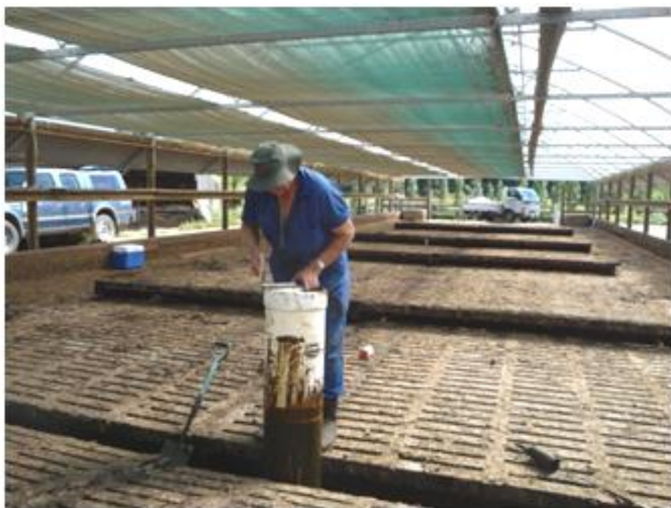
Photo 62: Specially designed PVC cylinder used for collecting samples. A handle at top of cylinder was used to homogenise manure within the cylinder before sampling.
