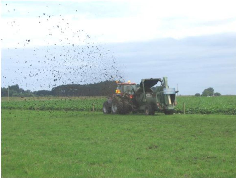
Photo 19: Manure solids being spread via side delivery orbital muck spreader.
