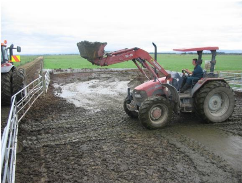
Photo 18: Feed pad scraped solids being loaded into muck spreader.
