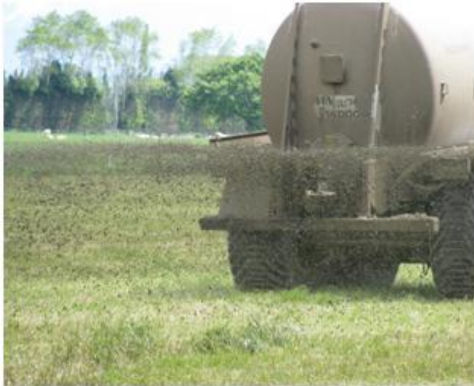
Photo 37: Rear delivery spreading pattern from slurry tanker.
