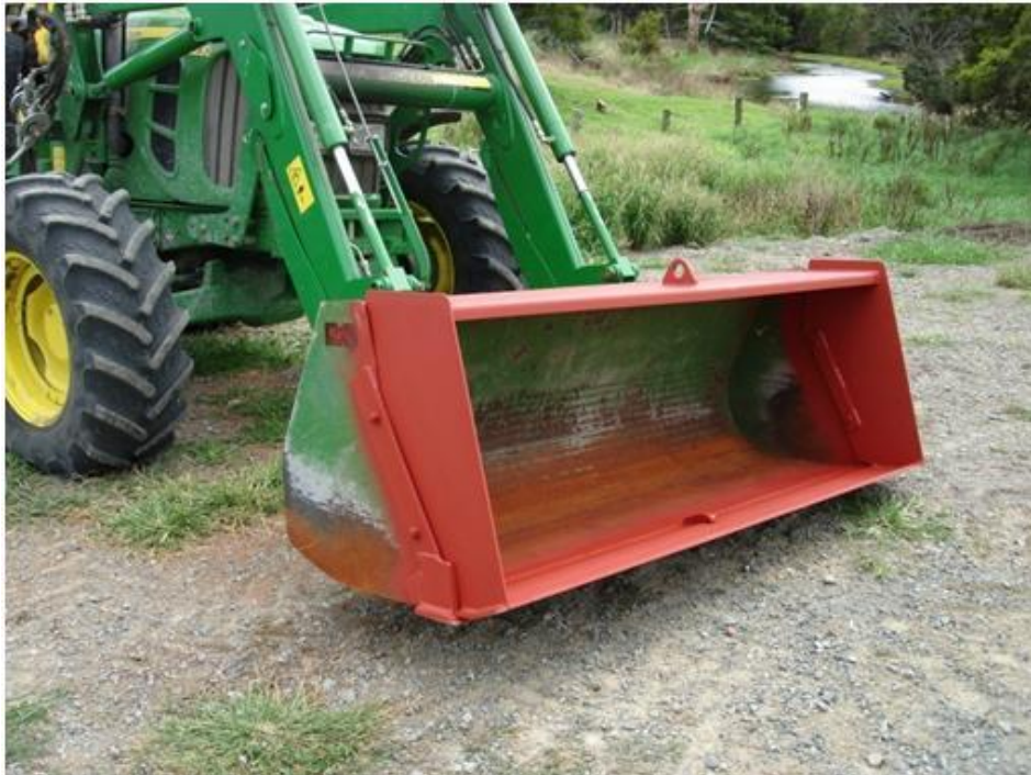
Photo 27: Modified bucket to reduce manure spillage when emptying bunkers.
