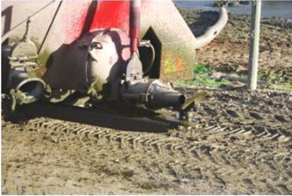
Photo 54: Rear delivery splash plate on the slurry tanker.
