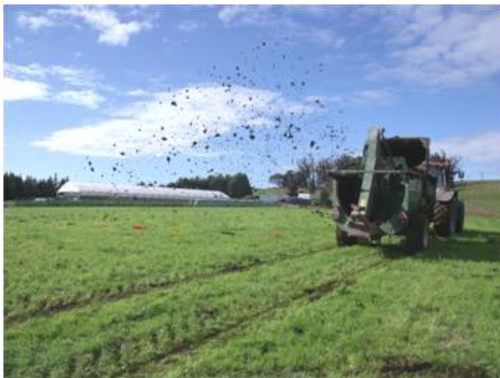
Photo 57: Side delivery of solids from orbital muck spreader.
