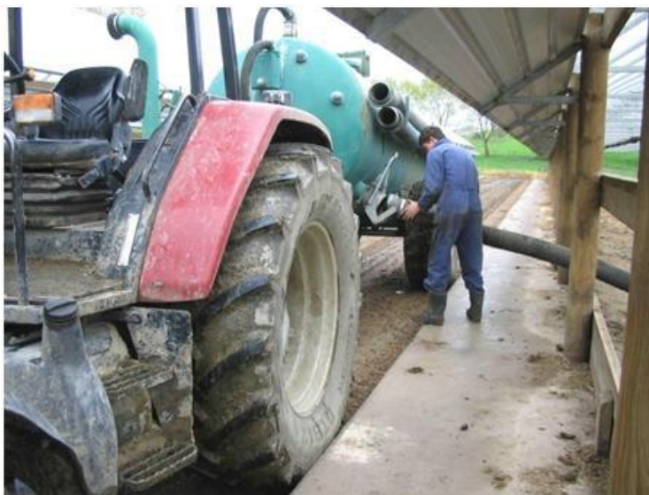
Photo 2: 15 cm diameter hose attached to slurry tanker for delivering slurry.
