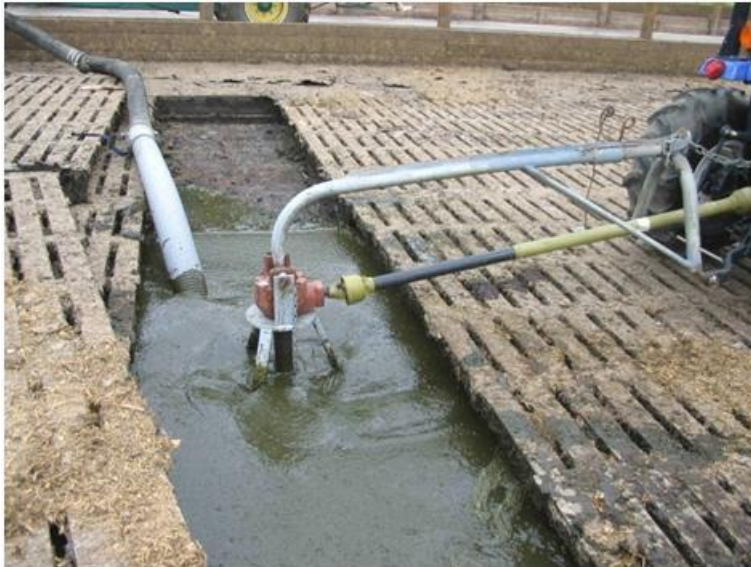
Photo 1: Vertical stirrer, designed by Richard Stewart, produces homogenous slurry in nearest bunker.
