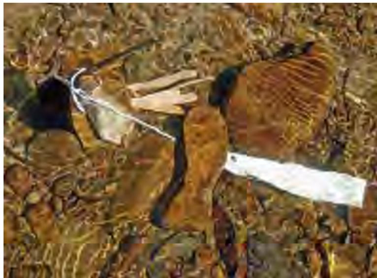
Figure 5.25: Wooden sticks and cotton strips deployed in-stream
