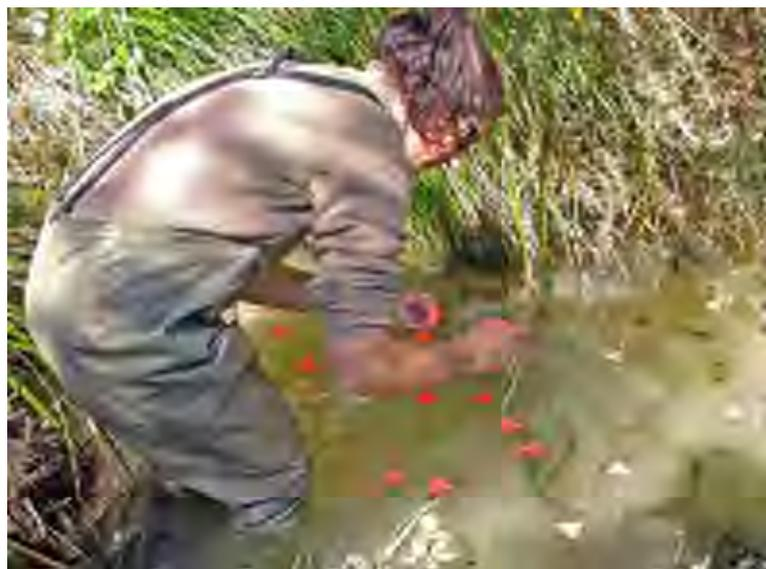
Figure 5.14: Release of waterproof paper triangles.
