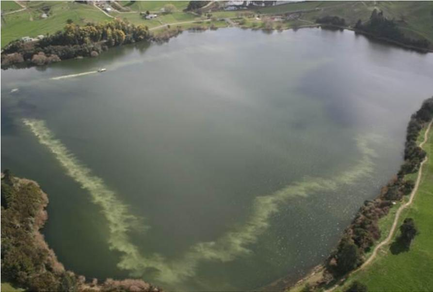
Figure 11 Aerial view of Aqual-P (modified zeolite) application in Lake Okaro, Bay of Plenty (Photo: Andy Bruere).
