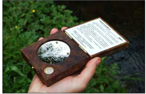
Figure 20. A spherical densiometer which is divided into 25 squares. Counting the number of squares with shading gives an accurate and repeatable estimate of the proportion of canopy cover over the reach.
