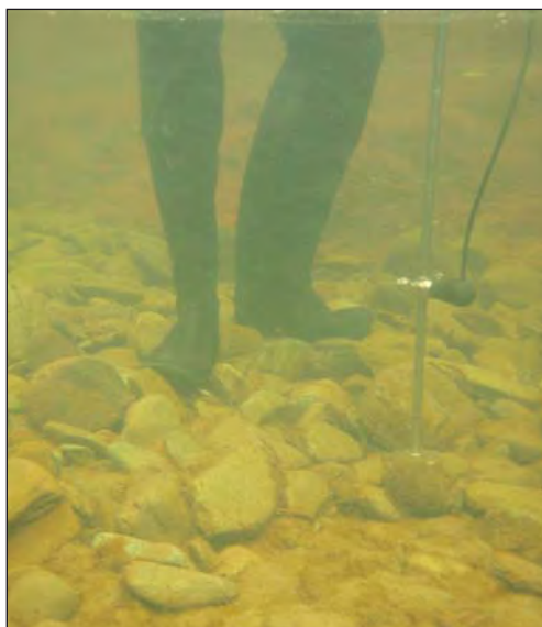
Figure 7. “Mean” water velocity is measured at four-tenths of water depth from the surface.
