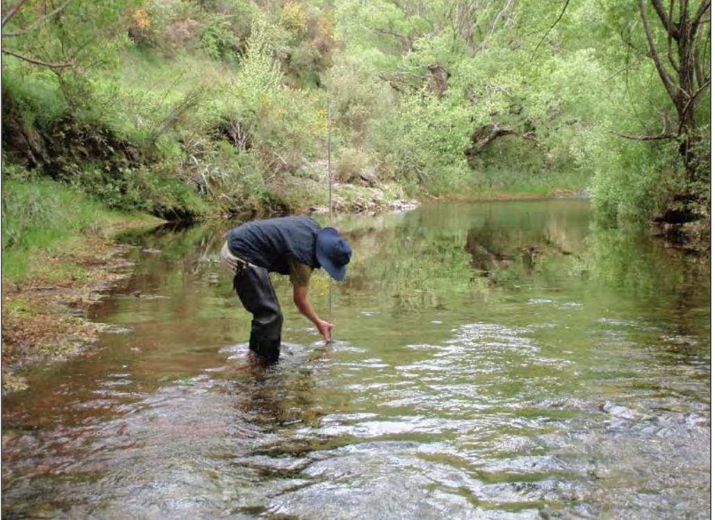
Figure 10. Residual pool depth is the water depth measured at the riffle crest immediately downstream of a pool subtracted from the depth at the deepest point in the pool.
