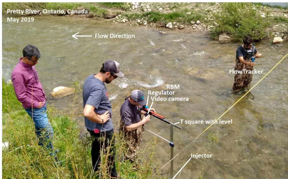
Figure E-1: Experimenting with an RBM wading rod and nitrogen bubbles in Pretty River, Ontario, Canada.
