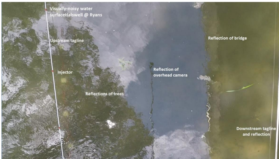
Figure 6-22: View from the right bank illustrating the visual challenges in recognising surfacing bubbles.
