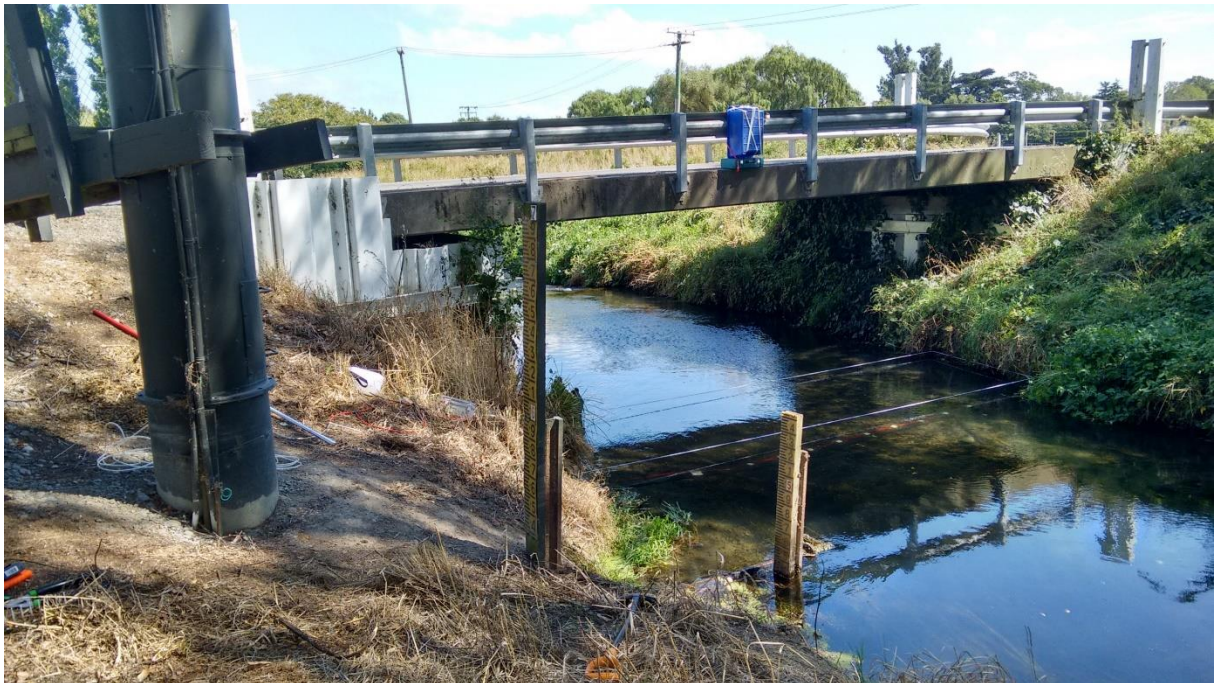
Figure 6-9: The reference site at Halswell showing taglines and prototype bubble line. The level to flow station stilling well is on the left.
