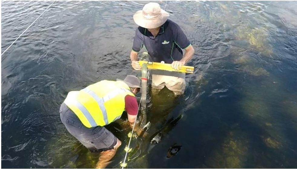
Figure 7-2: Aligning the bubble line with the tagline, using a T-square with levels.
