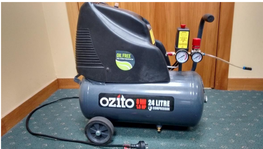
Figure B-2: Mains-powered compressor used at Halswell River where mains power is available.
