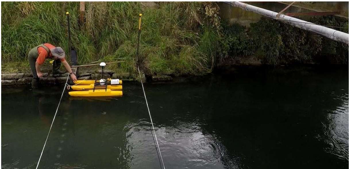
Figure 7-7: View from right bank. Deploying the ADCP boat (the reference) between the two taglines.
