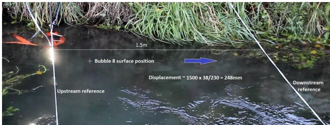
Figure 6-6: An early attempt to calculate displacement from each of the nine injectors
