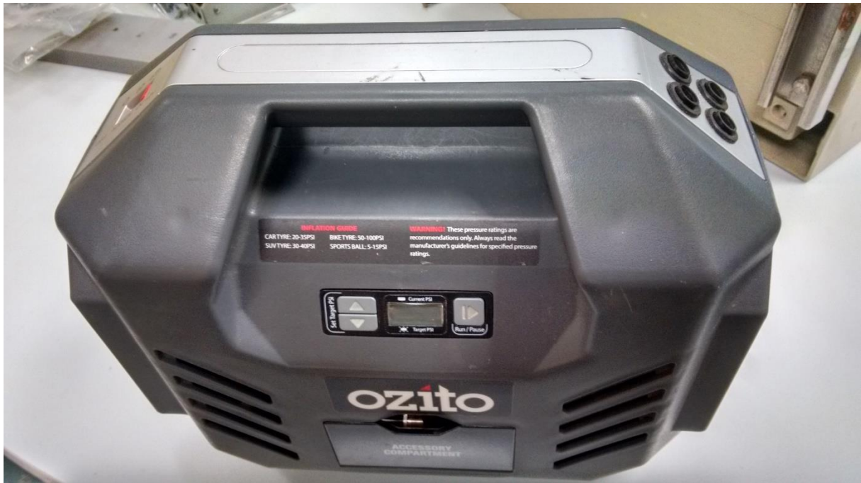
Figure B-3: This 12V DC battery (or 230V) powered compressor can pump up to 120 PSI but at low flow, so needs an external reservoir tank. We used a modified BBQ LPG tank. Being small and light
