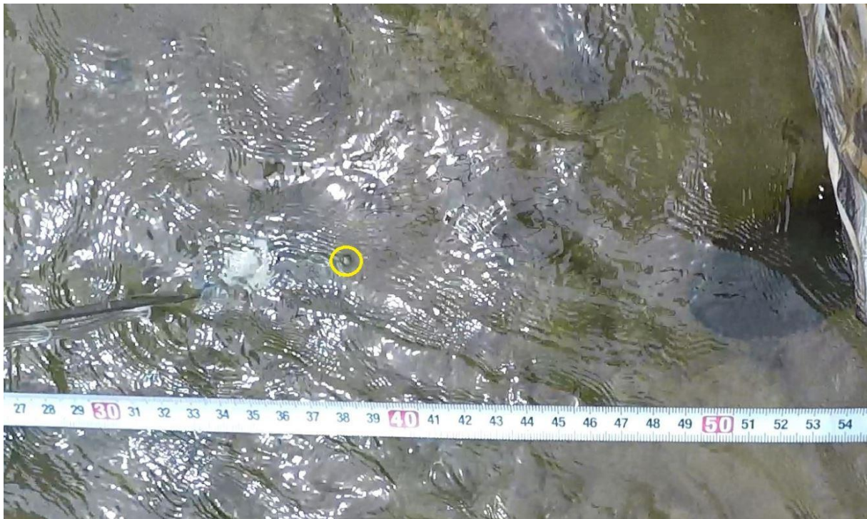
Figure E-2: The video frame in which a nitrogen bubble injected from the river bed just surfaces (annotated with yellow circle) - what the GoPro video camera saw. The measuring tape (used to measure displacement of the bubble) should have been closer to the water but the slider had jammed.
