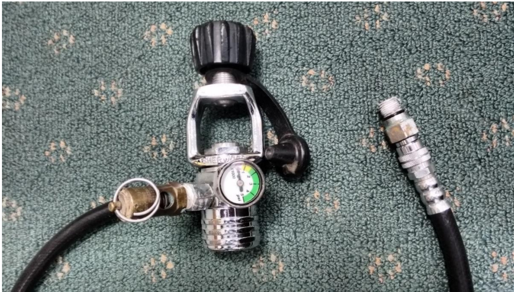
Figure B-1: The diver regulator we connected to the compressed air tank we used in early tests.
