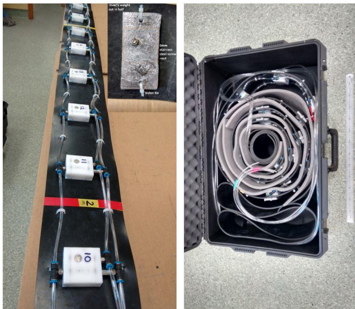
Figure 4-1: Left - 20-injector line assembled for HBRC; Right - the line rolled up in its carry case. It fits in the boot of an ordinary car. One person can carry it, but two are recommended, as with the lead ballast it weighs about 30 kg. Protective closed-cell foam has been rolled up with the bubble line.
