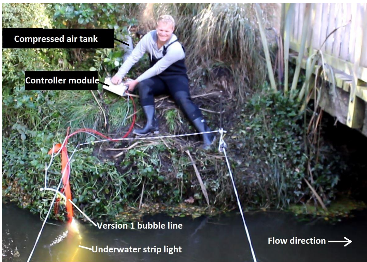
Figure 6-1: The very first attempt at RBM deployment. The steep slope made it hard to set up the taglines.
