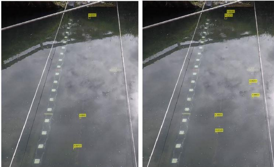
Figure 8-5: The AI bubble detector can now detect bubbles from the farthest injectors at the left bank.
