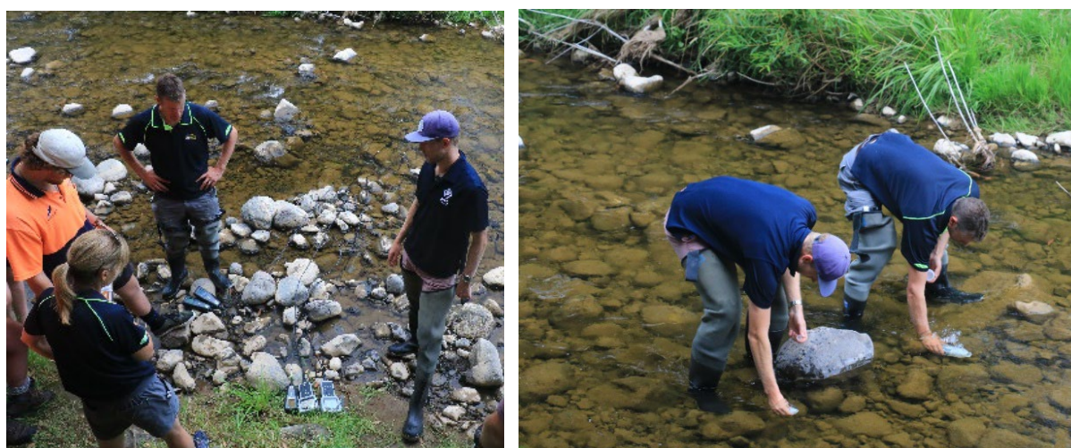
Figure 3-8: Monitoring officers from NIWA and Otago Regional Council carrying out side-by-side field measurements (left) and water sample collection (right). The two water samples were sent to the lab for nutrient analysis to check whether there was close agreement in the results (as would be expected). Photos: Juliet Milne.
