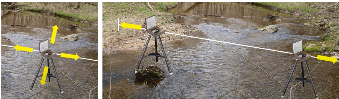
Densiometer set up for observations at mid-stream (A) and a single observation bankside (B). Photos: USWS.
